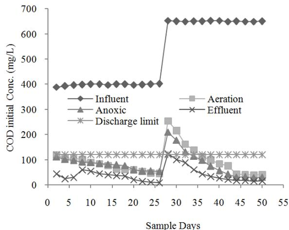
Fig. 1: COD removal in phases 1 and 2
