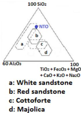
Fig. 10: Positioning of NTO sample in Fiori diagram (chemical composition) (Boch, 2001; Fiori *et al.*, 1989)
