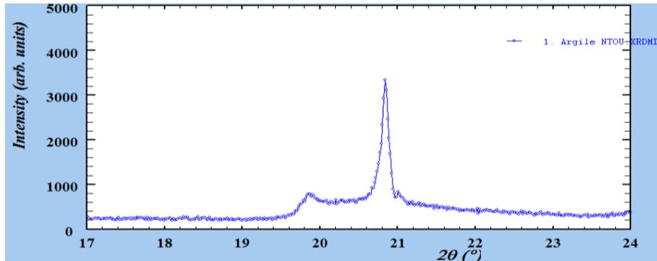
Fig. 9: NTO K<sub>2</sub>O sample in Ntokou diffractogram
