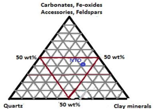
Fig. 11: Positioning of NTO sample in Fiori diagram (mineralogical composition) (Fiori *et al.*, 1989)
