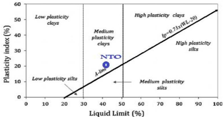
Fig. 6: Positioning of NTO sample in Casagrande chart (Casagrande, 1948)
