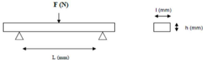
Fig. 1: Flexural strength
