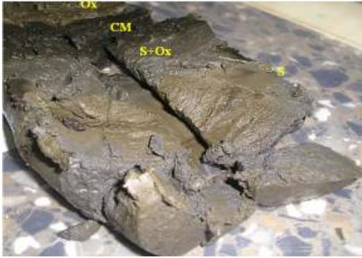
Fig. 1: Split tailings from a 15 cm core taken at 2 m from that shows stratification: S-sulfide and Ox- oxide and CM-carbonaceous material
