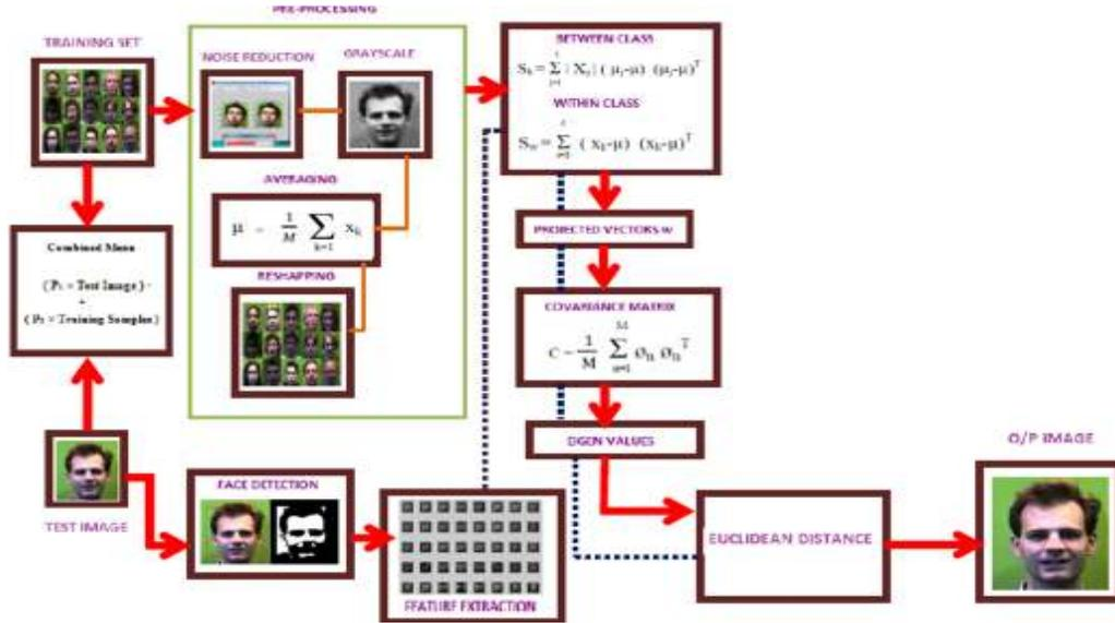
Fig. 3: Block diagram of LDA
