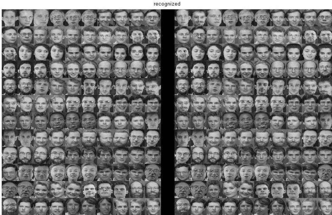
Fig. 14: ORL database-LDA MATLAB simulation output (120 test images given as input and the corresponding recognized image; Here eight image wrongly recognized. Hence we get a Recognition Rate =  $(112/120) \times 100 = 93.33\%$ ) for above sample as 120 test images we got recognition rate as 93.33%
