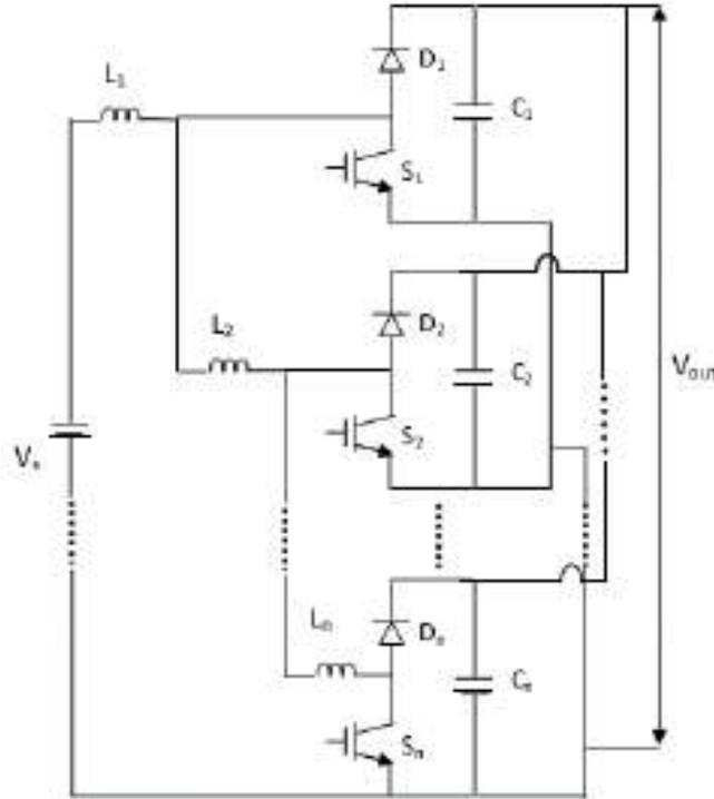
Fig. 1: Structure of cascade DC-DC boost converter
