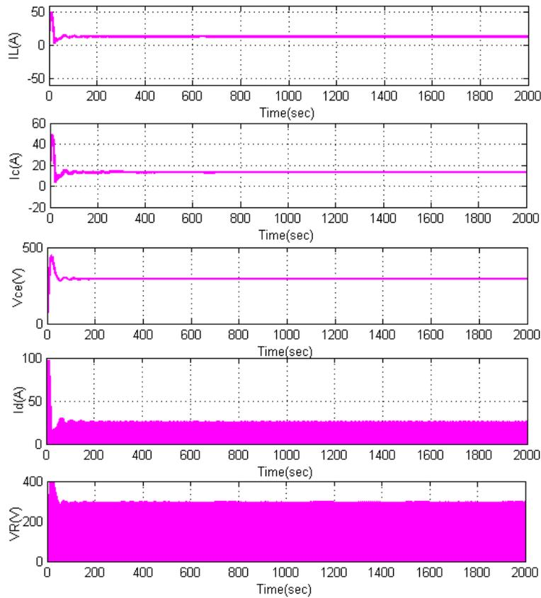
Fig. 9: Performance of inductor current ( $I_L$ ), capacitor current ( $I_C$ ), load voltage ( $V_{ce}$ ), diode current ( $I_d$ ) and IGBT switching voltage ( $V_R$ )
