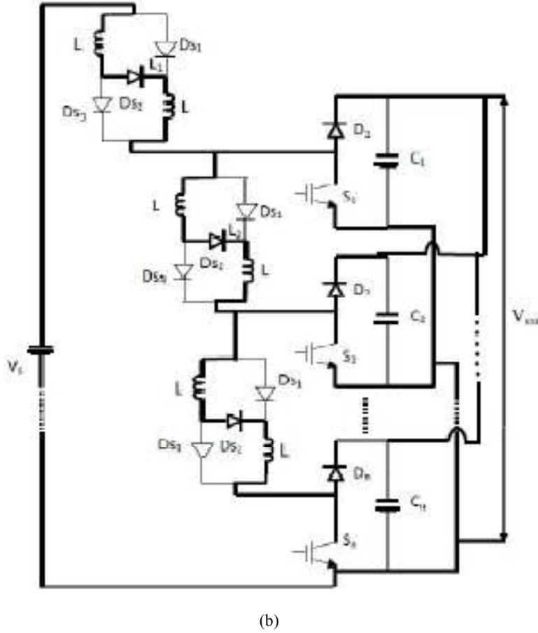
Fig. 4: H-bridge switched inductor base cascade dc-dc boost converter while (a) Mode I operation and (b) Mode II operation
