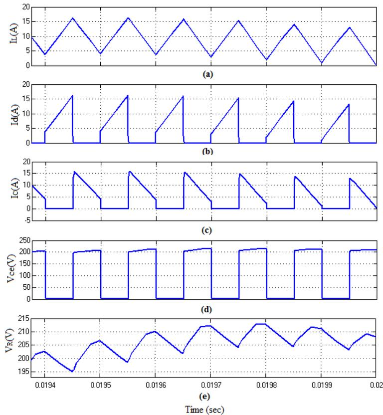
Fig. 6: Theoretical performance of; (a): Inductor current ( $I_L$ ); (b): Capacitor current ( $I_C$ ); (c): Diode current ( $I_D$ ); (d): Load voltage ( $V_{ce}$ ) and; (e): IGBT switching voltage ( $V_R$ )
