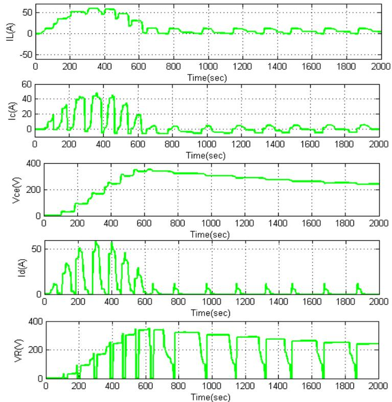
Fig. 8: Performance of inductor current ( $I_L$ ), capacitor current ( $I_C$ ), load voltage ( $V_{ce}$ ), diode current ( $I_d$ ) and IGBT switching voltage ( $V_R$ ) by multilevel dc-dc boost converter
