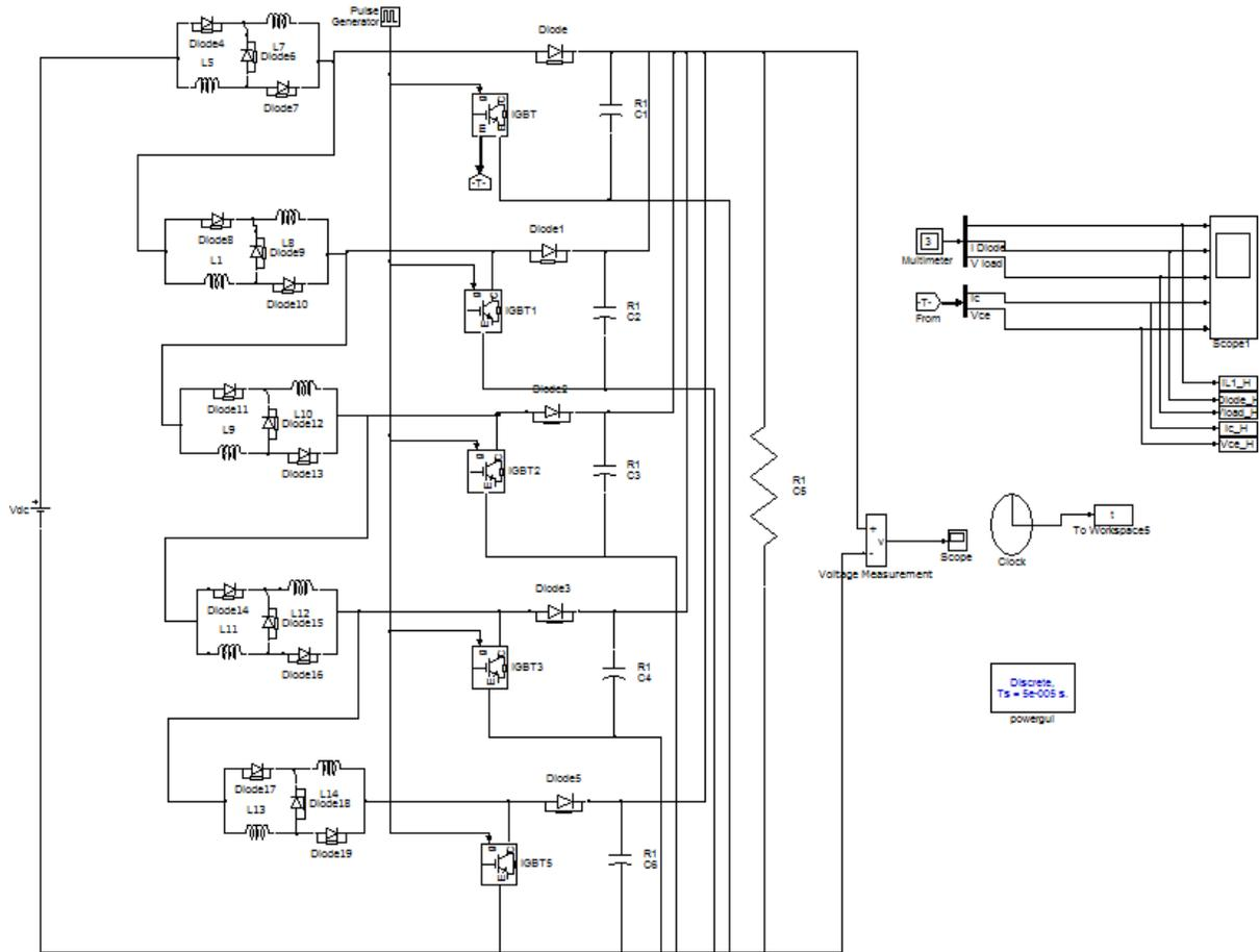
Fig. 5: Simulink model of H-bridge switched inductor with multilevel DC to DC boost converter topology
