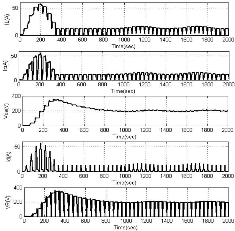
Fig. 7: Performance of inductor current ( $I_L$ ), capacitor current ( $I_C$ ), load voltage ( $V_{ce}$ ), diode current ( $I_d$ ) and IGBT switching voltage ( $V_R$ ) by single level dc-dc boost converter
