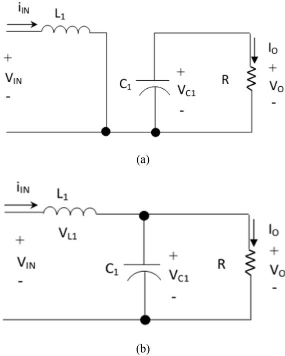
Fig. 2: Equivalent circuit of (a) switch-ON and (b) switch-OFF
