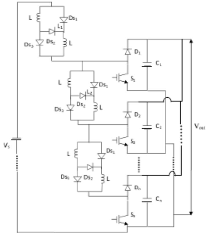
Fig. 3: Proposed H-bridge switched inductor base cascade dc-dc boost converter
