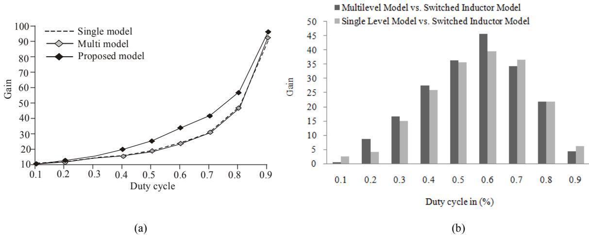
Fig. 11: Comparison Performance of (a) Voltage gain and duty cycle and (b) Deviation of switched inductor model
