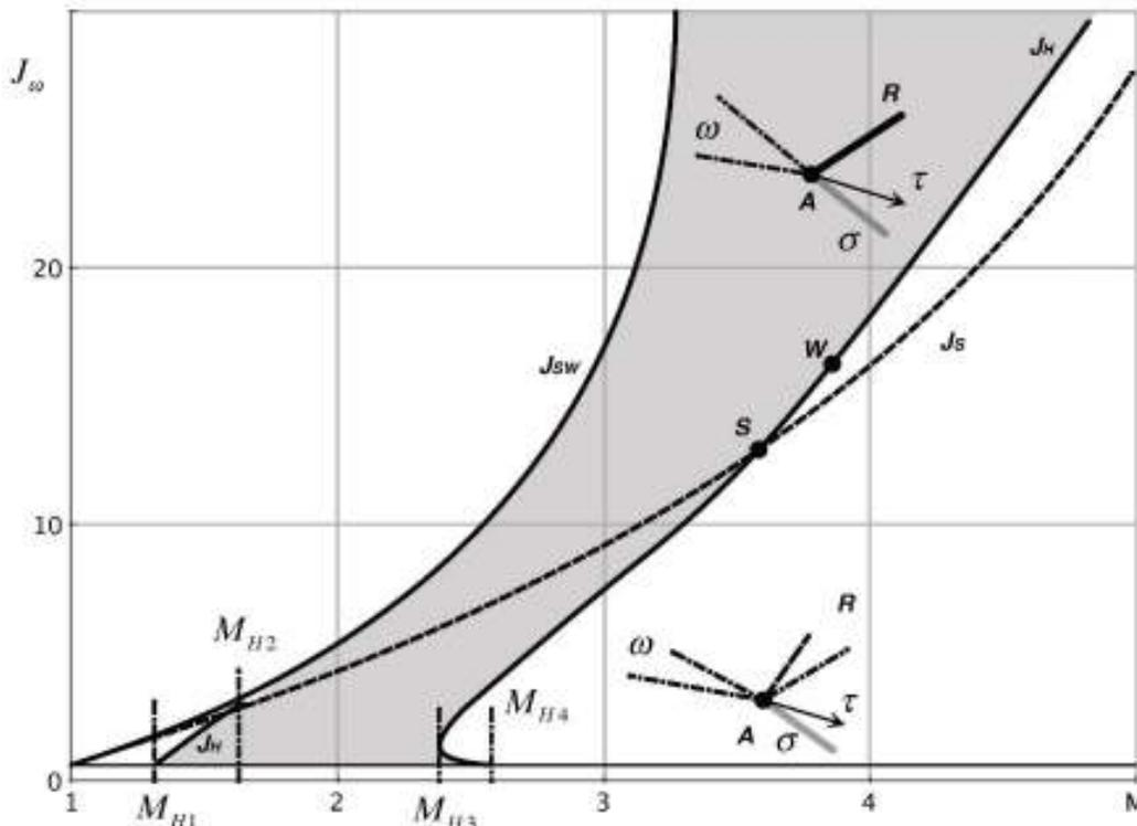
Fig. 5: Neutral polar and domain of CCW existence with reflected discontinuity-shock (shaded)  $J_\omega$  is the intensity of the centered compression wave,  $J_{sw}$  is the sound intensity of the centered compression wave,  $J_s$  is the sound intensity of shock,  $M_{1-4}$  are the special Mach numbers,  $M_w$  is the Mach number limiting the domain of existence of shockwave structures with reflected discontinuity-shock
