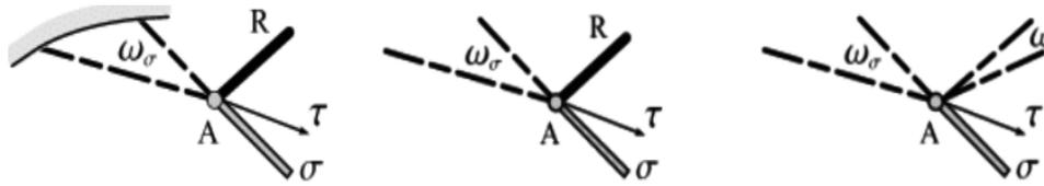
Fig. 1: Centered compression wave; a): Common case; b): Reflected discontinuity-shock; c): Reflected discontinuity-centered depression wave
