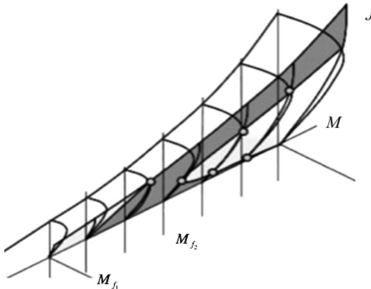
Fig. 3: Transformation of polars according to change of the Mach number the compression polar is toned, the shockwave is transparent
