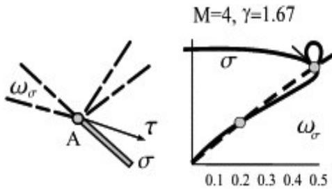
Fig. 7: Polars meeting the “special Mach number  $M_w$ . At  $M > M_w$  SWS with reflected discontinuity-a shock cannot exist
