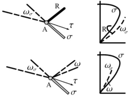
Fig. 2: CCW with reflected discontinuity shock and depression wave
