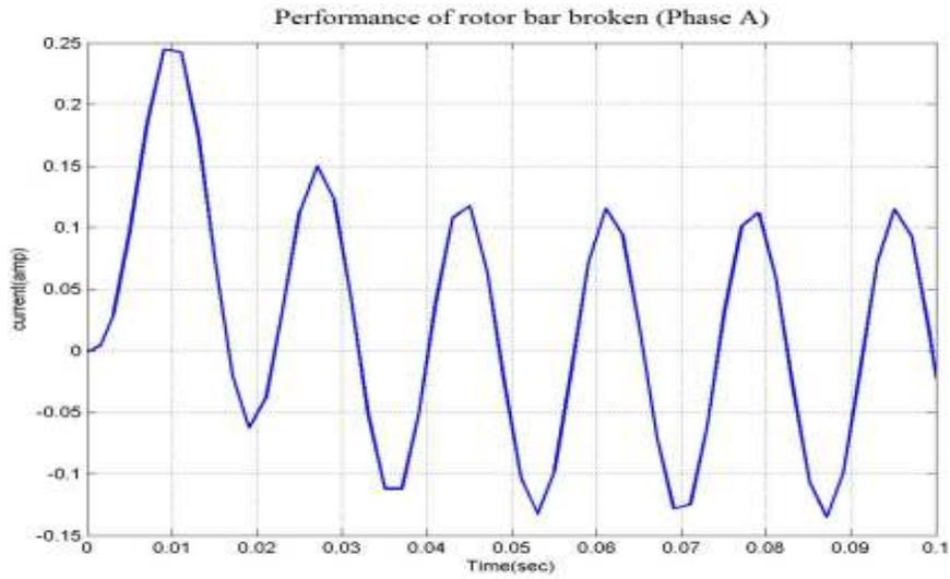
Fig. 4: Stator current for induction motor with broken rotor bar
