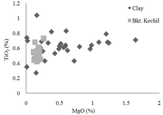
Fig. 7: Dry weight percentage (%) of the MgO and TiO<sub>2</sub> elements for the brick samples of candi bukit kechil and clay at Bujang valley
