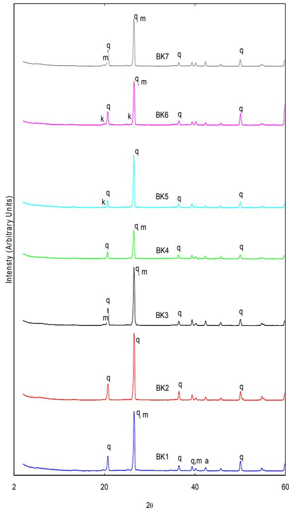
Fig. 3: The XRD diffraction pattern of candi bukit kechil bricks
