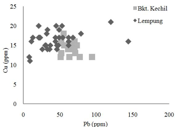
Fig. 8: Graph of lead and copper element concentration for the brick samples of candi bukit kechil and clay at Bujang valley
