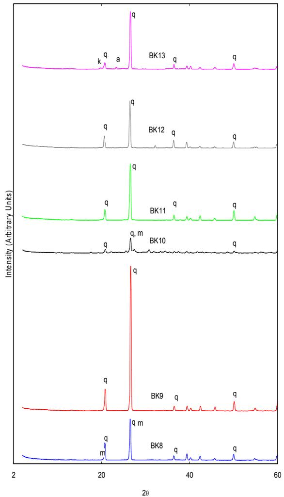
Fig. 4: XRD diffraction pattern of candi bukit kechil bricks
