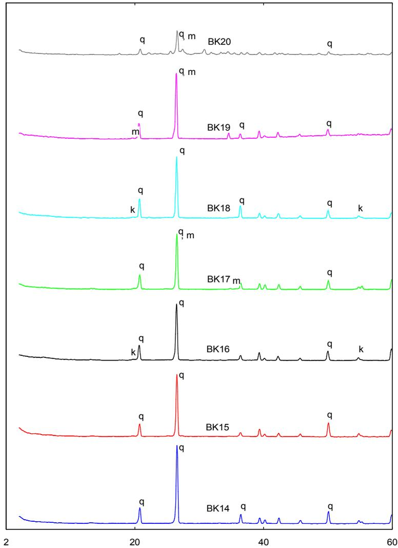
Fig. 5: XRD diffraction pattern of candi bukit kechil bricks
