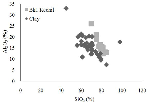
Fig. 6: Dry weight percentage (%) of the elements SiO<sub>2</sub> and Al<sub>2</sub>O<sub>3</sub> for the brick samples of candi bukit kechil and clay at Bujang valley
