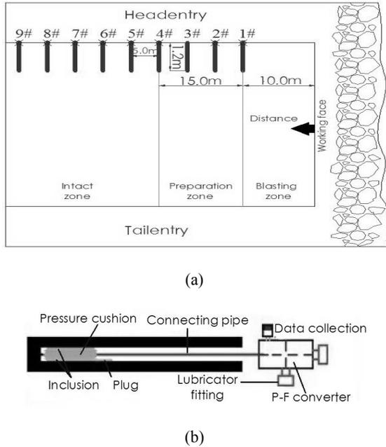
Fig. 7: In-situ monitoring conditions; (a): Layout of general in-situ monitoring; (b): Stress monitoring principle and field data acquisition
