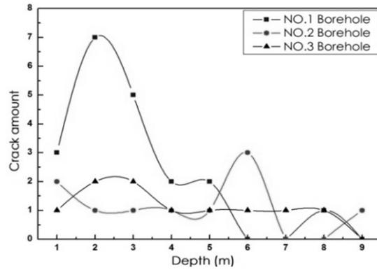
Fig. 6: Statistical regularity of cracks with advent of borehole depth
