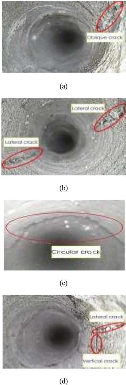
Fig. 5: All kinds of borehole cracks (a): Oblique crack; (b): Lateral crack; (c): Circular crack; (d): Lateral crack and vertical crack
