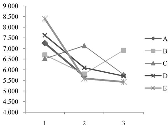
Fig. 2: Effect of cutting parameters on mean value S/N ratio for surface roughness
