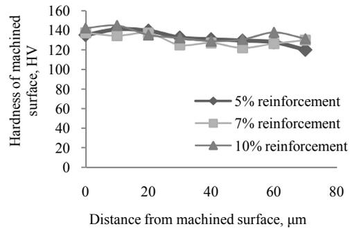
Fig. 3: Effect of percentage of reinforcement on microhardness variations for AISi/AlN MMC
