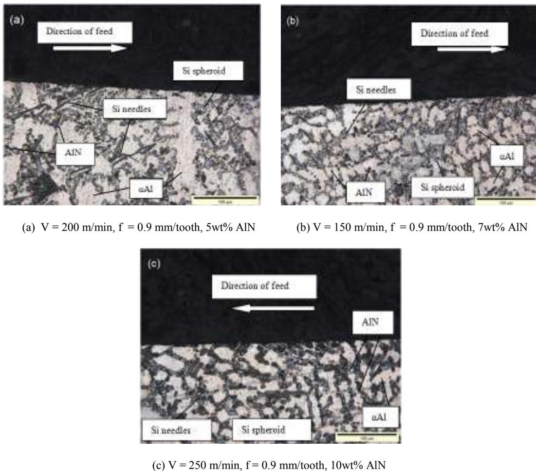
Fig. 4: Microstructure of AlSi/AlN MMC for different cutting condition
