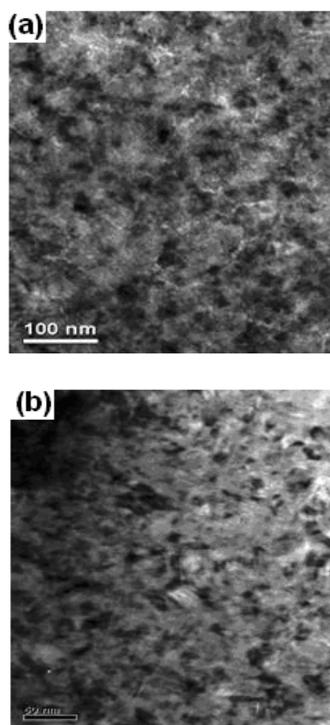
Fig. 3: Surface morphology of Ni-TiN nanocomposite layer obtained by ultrasonic electrode position at a scale of: (a) 100; and (b) 50 nm
