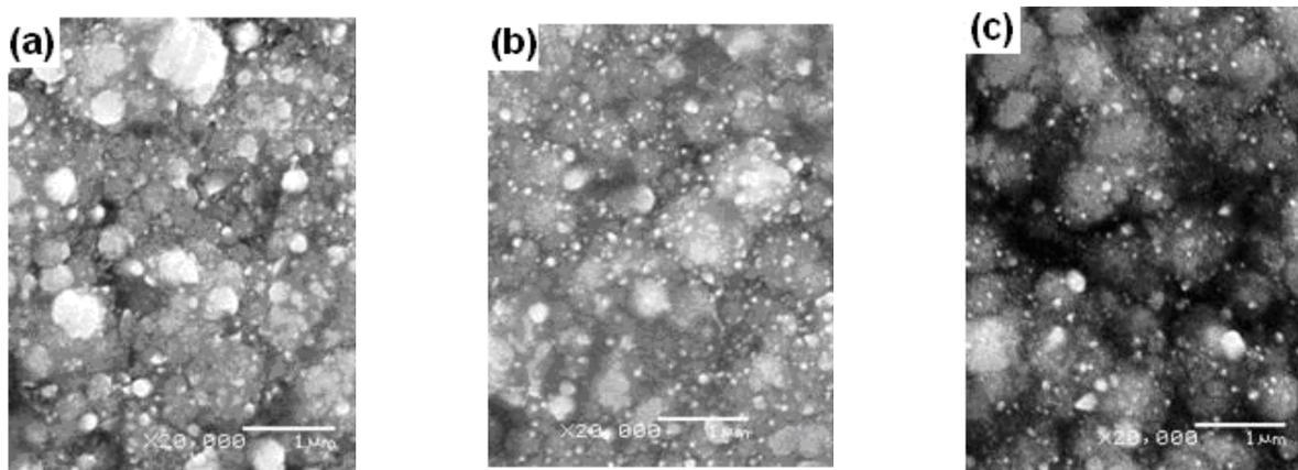
(a) Mechanical stirring, no ultrasonication (b) Moderate ultrasonication (200 W) (c) Strong ultrasonication (300 W)
