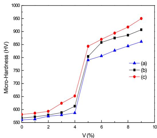
Fig. 4: The effect of V on micro-hardness of Ni-TiN composite layers deposited under different ultrasonic power (a) Mechanical stirring, no ultrasonication; (b) Moderate ultrasonication (200 W); (c) Strong ultrasonication (300 W)
