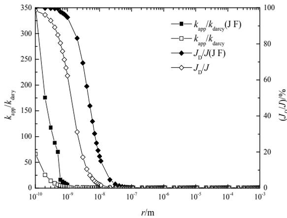
Fig. 4: The ratio of the methane apparent permeability to Darcy permeability and diffusion flux to total mass flux with the different pore radius (350 K, 5MPa)
