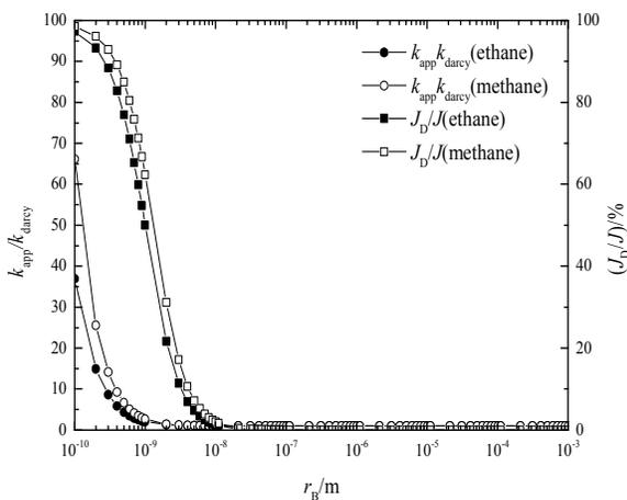
Fig. 5: The ratios of the methane and ethane apparent permeability to the Darcy permeability and diffusion flux to total mass flux with the different pore radius (350 K, 5 MPa)
