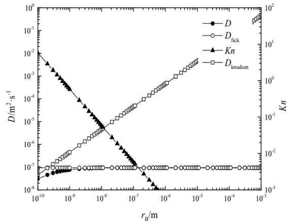
Fig. 2: The methane diffusion coefficient in different pore radius (300K, 5MPa)
