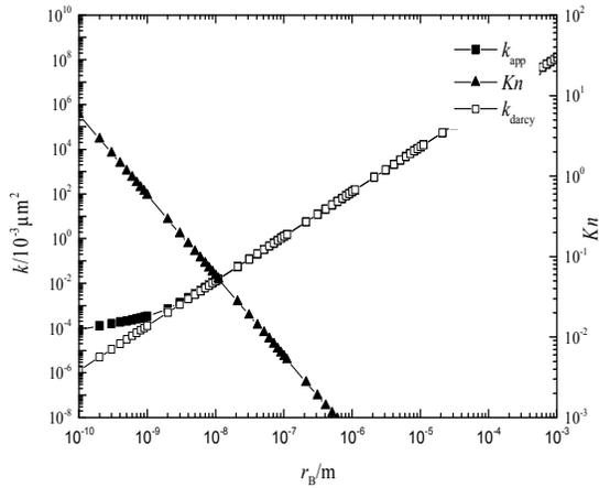
Fig. 3: The methane apparent permeability with the different pore diameter (350 K, 5MPa)
