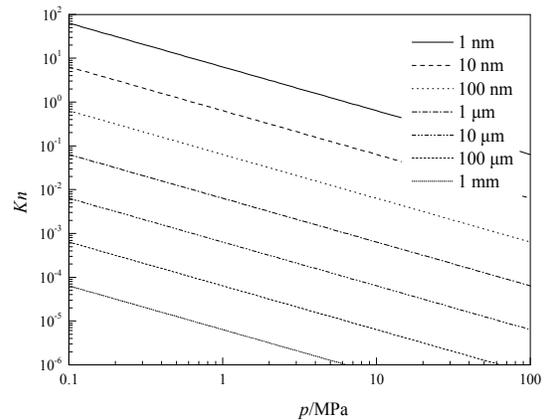
Fig. 1: The trends of  $Kn$  number with the different pore diameter and pressure (350 K)
