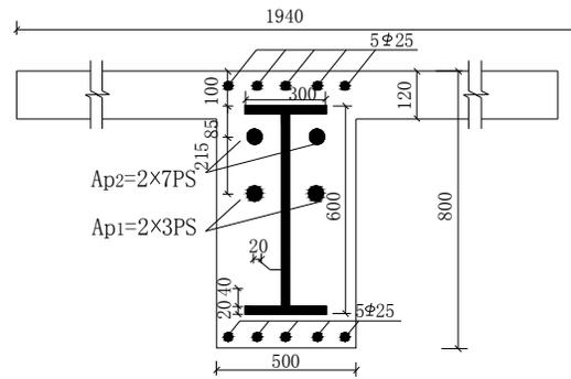
Fig. 10: Section of encased H-shape steel prestressed concrete composite frame beams at support
