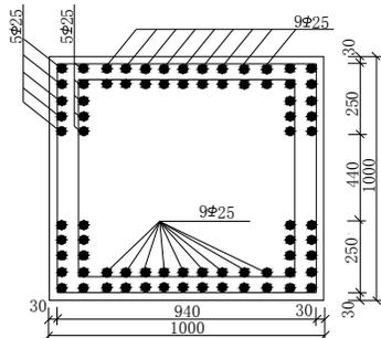
(b) Equivalent reinforced concrete column
