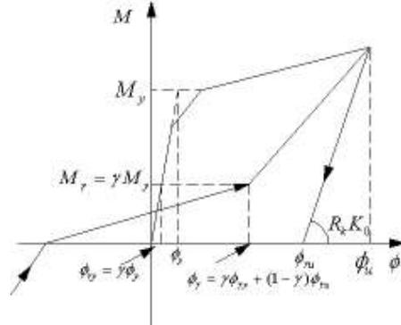
Fig. 7: Slip and pinch degradation
