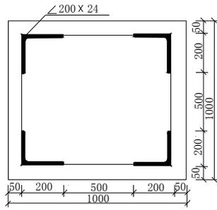
(a) Angle steel concrete column
