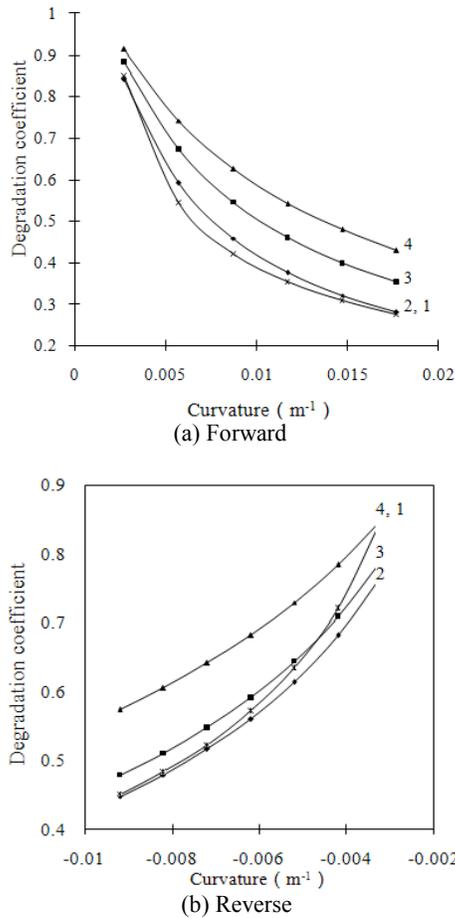
Fig. 11: Stiffness degradation coefficient curves of frame beams
