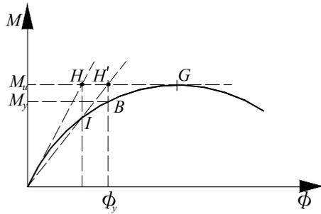
Fig. 9: Determination of yield point using current yield moment method
