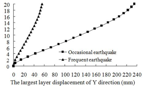
Fig. 7: The largest layer disp. of Y direction (mm)
