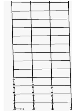
Fig. 10: The plastic hinge of structure
