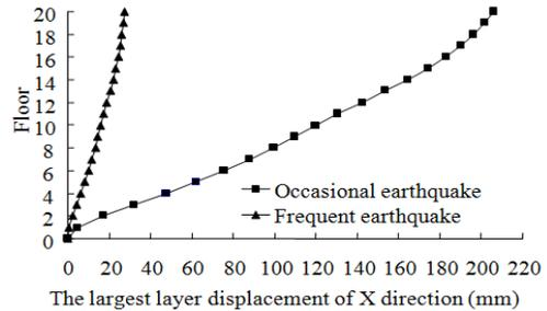
Fig. 6: The largest layer disp. of X direction (mm)
