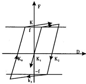
Fig. 1: Restoring force model
