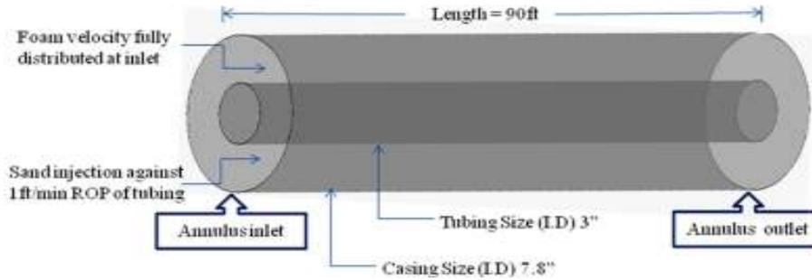
Fig. 4: Schematic well diagram
