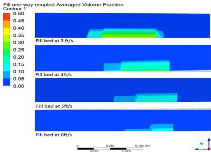
Fig. 13: Fill bed along bottom of the annulus for 90% quality foam
