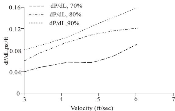
Fig. 14: Annular pressure gradient vs. flow velocity
