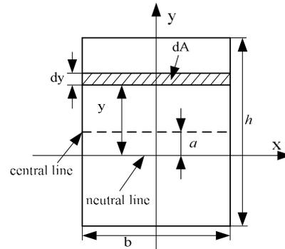
Fig. 4: Cross section of rectangular archwire
