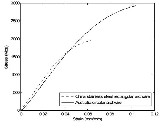
Fig. 6: Stress-strain curve of archwire
