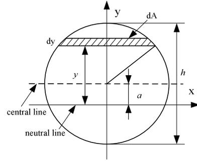
Fig. 5: Cross section of circular archwire
