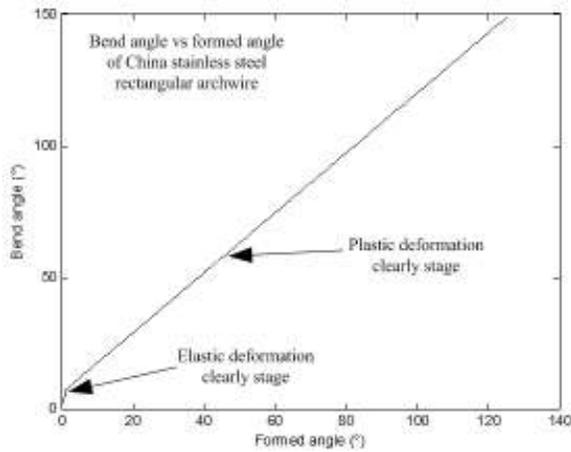
Fig. 7: Theoretical curve of bend angle vs formed angle of China stainless steel rectangular archwire
