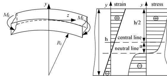
Fig. 3: Relationship of stress and strain with neutral line shift
