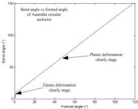
Fig. 8: Theoretical curve of bend angle vs formed angle of Australia circular archwire
