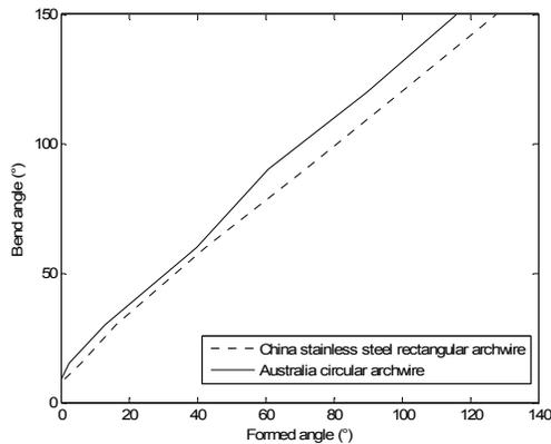
Fig. 12: Experimental curve of bend angle vs formed angle of two archwires
