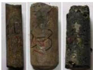
Fig. 2: Epoxy-repaired rocks
