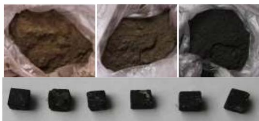
Fig. 3: Sample preparation for XRD and SEM tests
