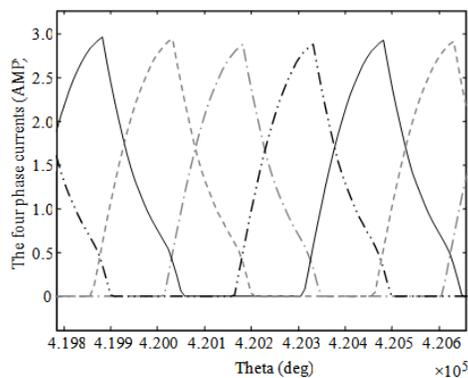
Fig. 12: The four phase instantaneous stator current at high speed with variable load torque
