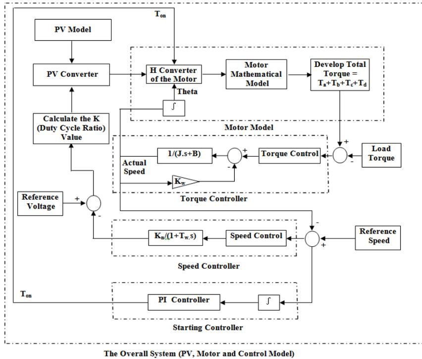
Fig. 4: Simplified model and control system for SRM
