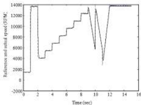
Fig. 11: Actual and reference speed versus time for variable and pump loads
