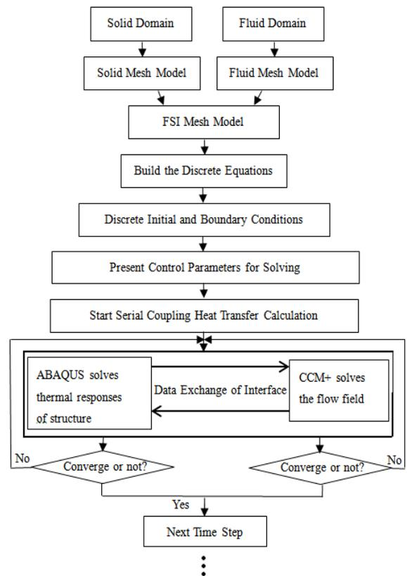
Fig. 1: Flow chart of transient heat transfer
