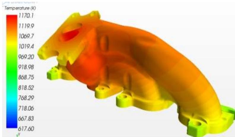
Fig. 8: Steady temperature calculation result
