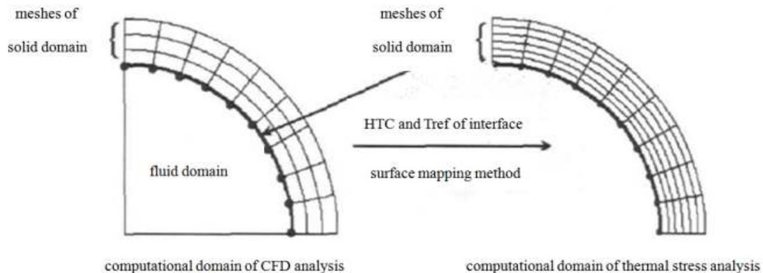
Fig. 6: Schematic diagram of surface mapping method
