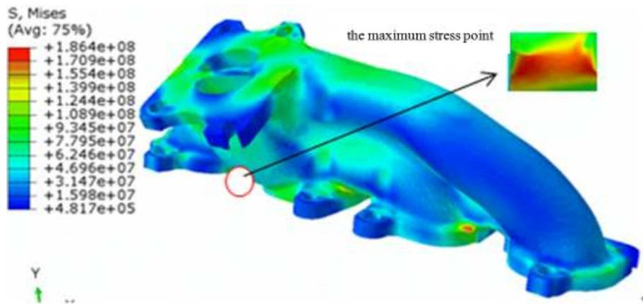
Fig. 11: Transient thermal stress calculation result (t = 905s)
