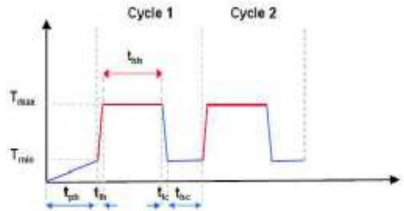
Fig. 5: Exhaust manifold temperature variation curve
