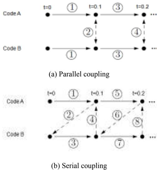
Fig. 2: Coupling mode of STAR-CCM+ and ABAQUS
