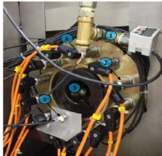
Fig. 2: Housing with pressure and temperature sensors. (1) Temperature sensor (2) Pressure sensor (3) Shaft (4) Temperature inlet (5) Temperature outlet
