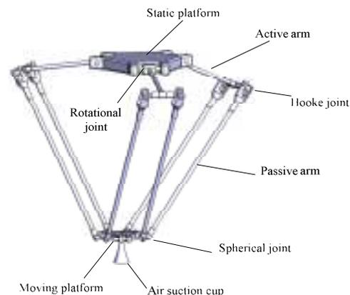
Fig. 1: 3-D model of 3-R2H2S parallel robot
