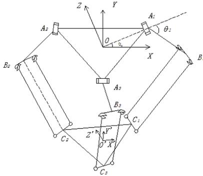
Fig. 2: Structure diagram of 3-R2H2S mechanism
