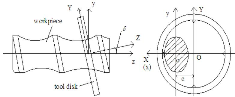
Fig. 2: Schematic diagram of whirling process
