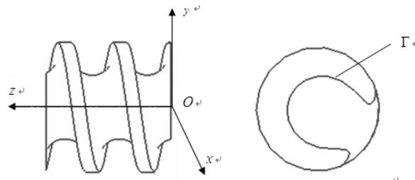
Fig. 1: Example of helical groove and its generatrix
