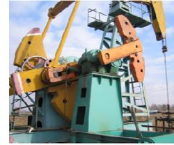
Fig. 4: Secondary balance device
