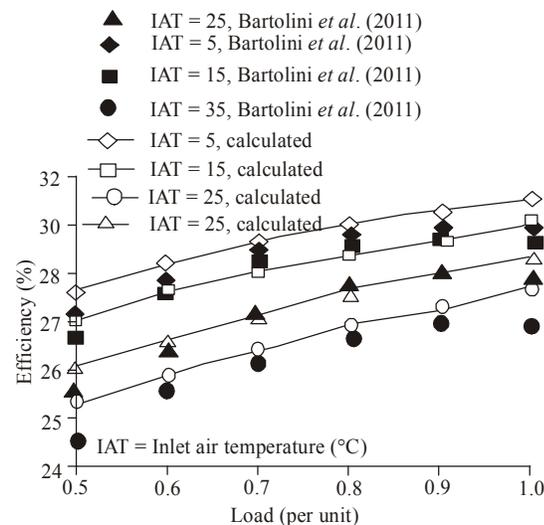
Fig. 4: Part-load efficiency in various ambient temperatures
