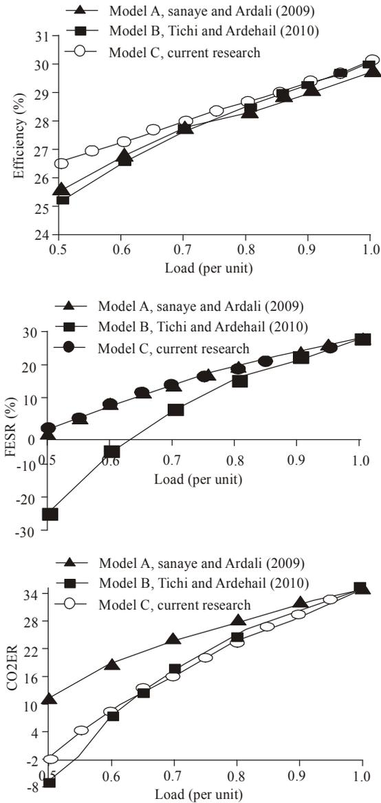
Fig. 5: Part-load effects on system
