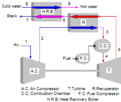
Fig. 1: Schematic diagram of a microturbine-based cogeneration plant
