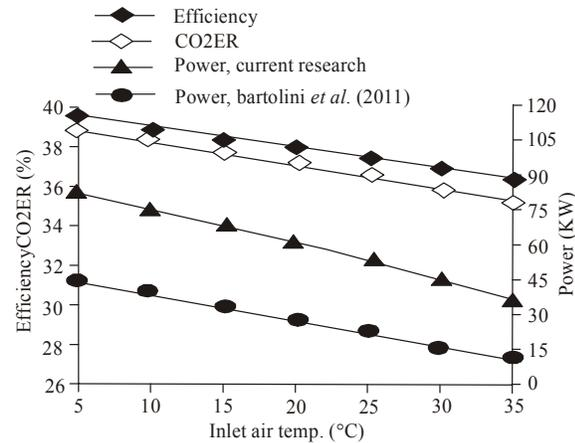
Fig. 3: Ambient temperature effects on system
