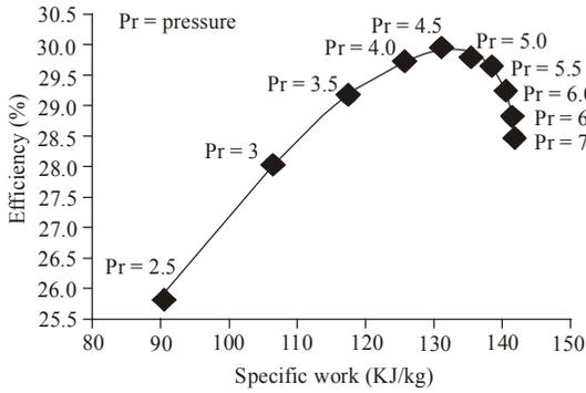
Fig. 2: Performance characteristic curve of microturbine
