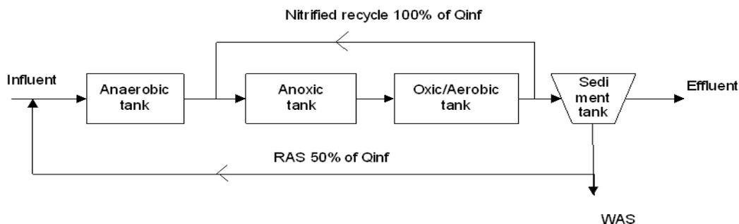
Fig. 3: Changzhou WWTP simplified schematic flow diagram
