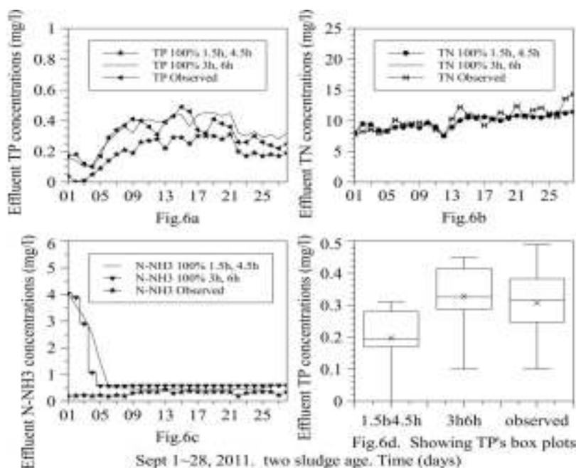
Fig. 6: a~d Effluent TP, TN and N-NH<sub>3</sub> concentrations for two sludge age; 100% 1.5 h 4.5 h = 100% internal recycle with the wastage pump on for 1.5h and then off for 4.5 h 100% 3 h 6 h = 100% internal recycle with the wastage pump on for 3 h and then off for 6 h)
