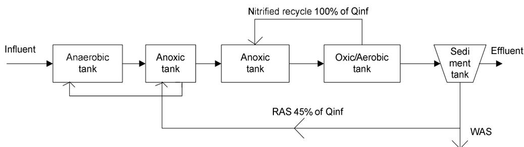
Fig. 4a: Nanjing WWTP simplified schematic flow diagram
