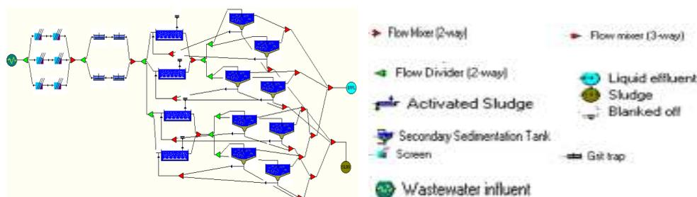
Fig. 4b: STOAT configuration of Nanjing WWTP
