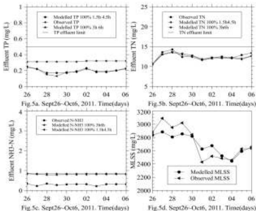
Fig. 5: a~d Effluent TP, TN, N-NH<sub>3</sub> concentrations and MLSS concentration in the tank; 100% 1.5 h 4.5 h = 100% internal recycle with the wastage pump on for 1.5 h and then off for 4.5 h 100% 3 h 6 h = 100% internal recycle with the wastage pump on for 3 h and then off for 6 h
