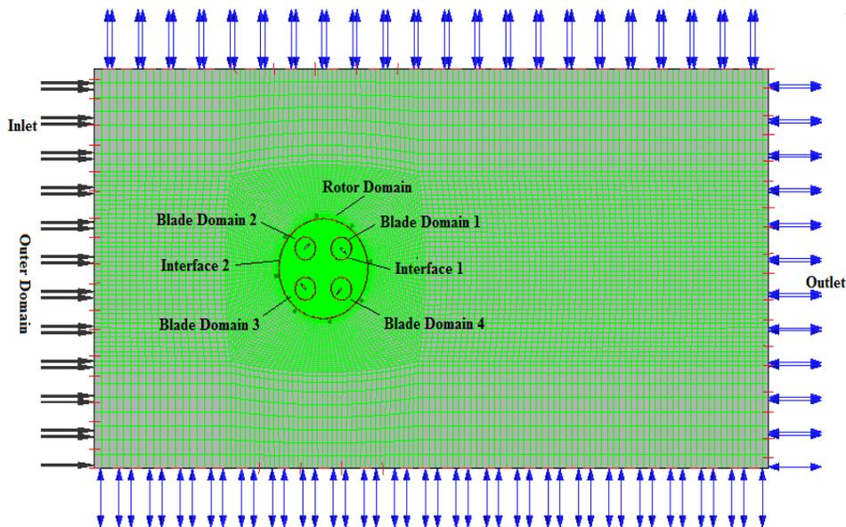
Fig. 8: Variable pitch simulation model
