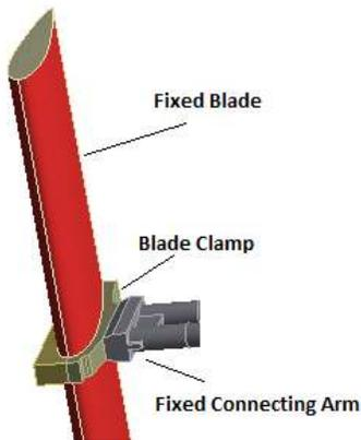
Fig. 4: Fixed blade turbine geometry
