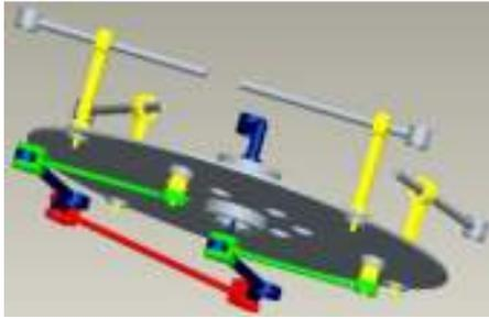
Fig. 2: Active variable pitch control mechanism
