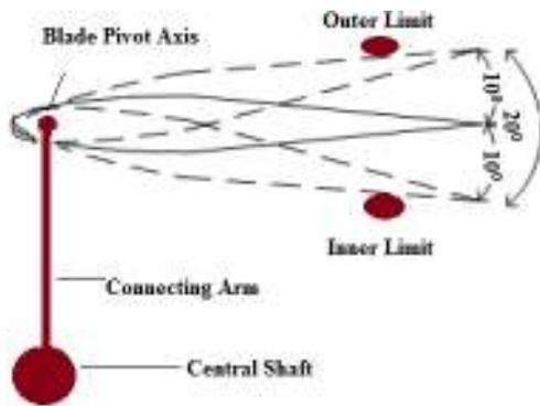
Fig. 3: Variable blade pitch angle position
