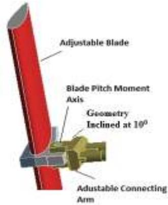
Fig. 5: Passive variable pitch geometry
