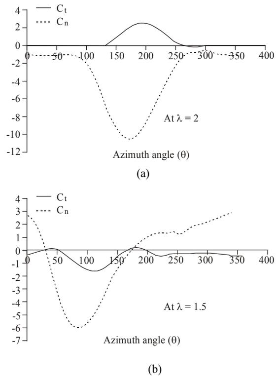
Fig. 10: Tangential & normal force coefficient vs. azimuth angle, (a) fixed pitch, (b) variable pitch
