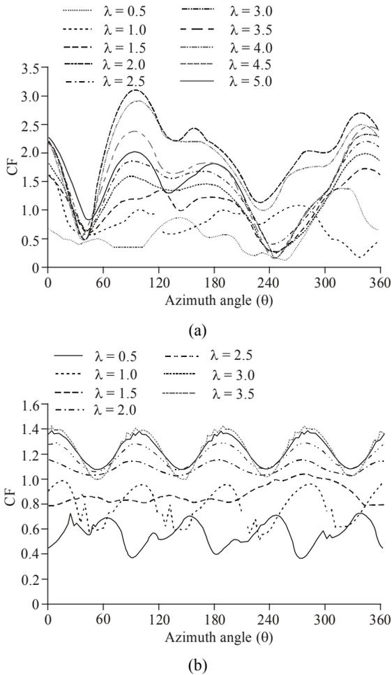
Fig. 9: Combined force coefficient for four blades vs. azimuth angle ( $\theta$ ), (a) fixed pitch, (b) variable pitch
