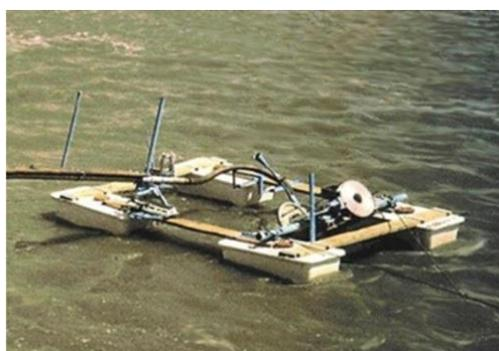
Fig. 19: Garman turbine: ITDG, model
