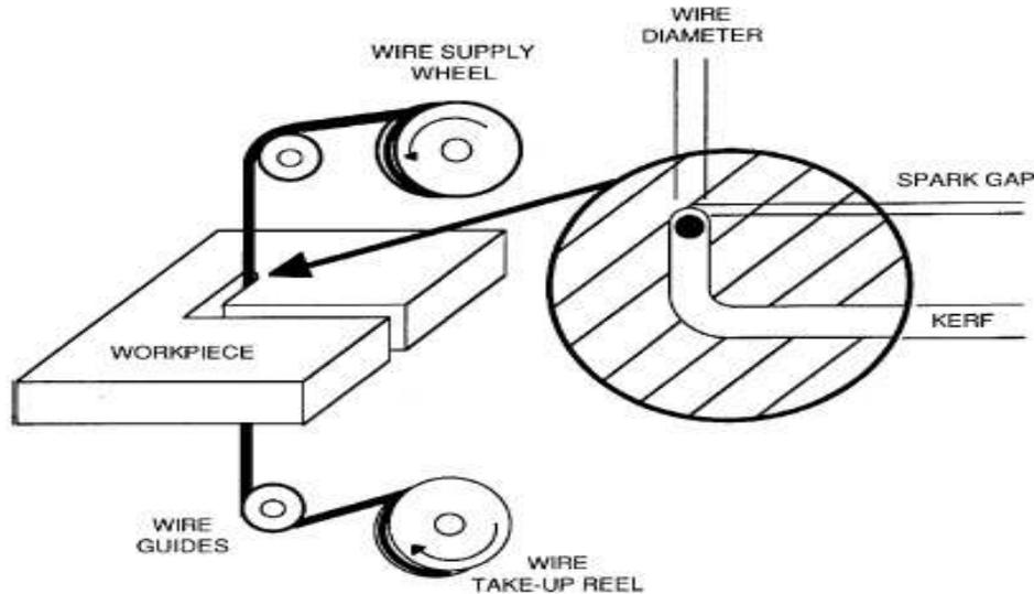
Fig. 1: Details of sparking gap (Scott *et al.*, 1991)
