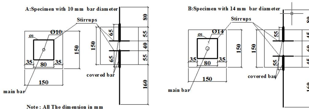
Fig. 1: The pullout reinforced casting specimen details
