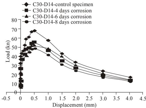
Fig. 8: Load and displacement relationship for C30-D14 specimen with different corrosion duration
