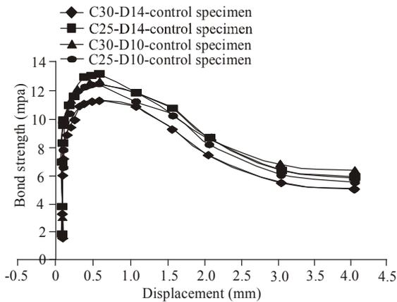
Fig. 11: Relationship between bond strength and displacement for control specimen
