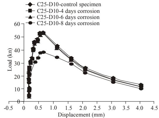
Fig. 9: Load and displacement relationship for C25-D10 specimen with different corrosion duration
