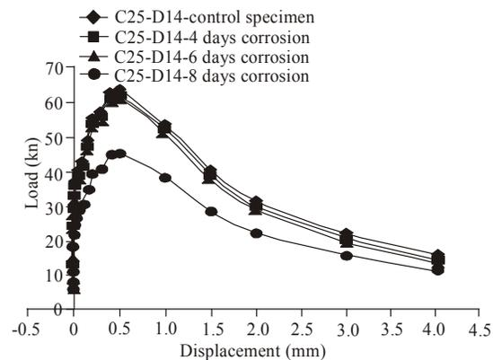
Fig. 10: Load and displacement relationship for C25-D14 specimen with different corrosion duration
