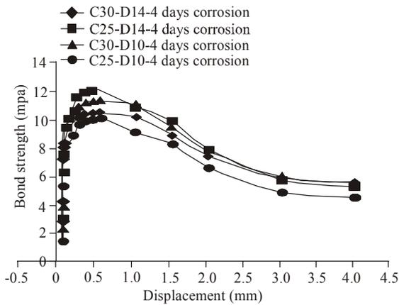
Fig. 12: Relationship between bond strength and displacement for 4 days corrosion specimen
