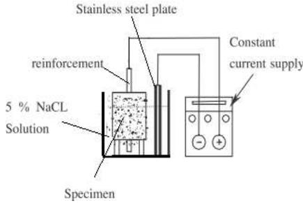
Fig. 2: The electrochemical acceleration system
