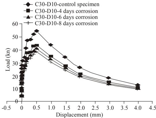
Fig. 7: Load and displacement relationship for C30-D10 specimen with different corrosion duration
