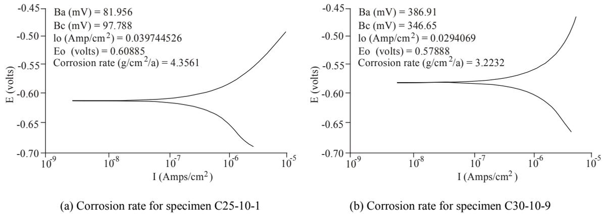
Fig. 4: The corrosion test result by using electrochemical measurement system (CS)
