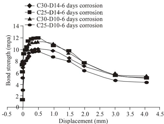
Fig. 13: Relationship between bond strength and displacement 6 days corrosion specimen
