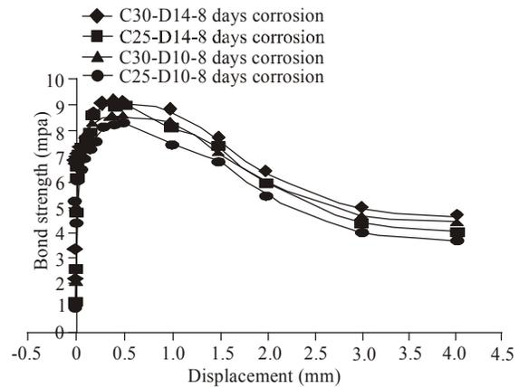
Fig. 14: Relationship between bond strength and displacement for 8 days corrosion specimen
