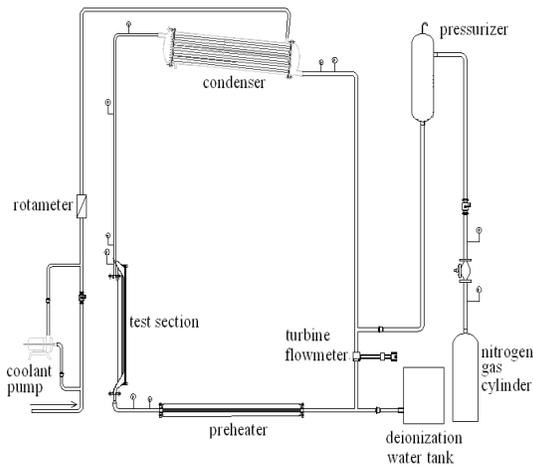
Fig. 1: Experimental loop of natural circulation
