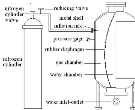
Fig. 3: Schematic diagram of pressurizer system
