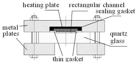
Fig. 2: Structure of test section
