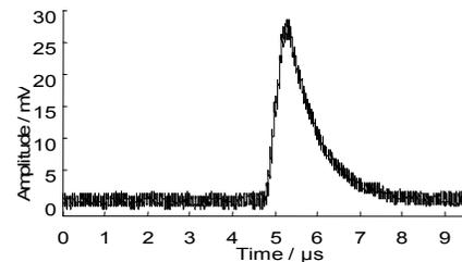
Fig. 5: Negative PD optical pulse in transformer oil
