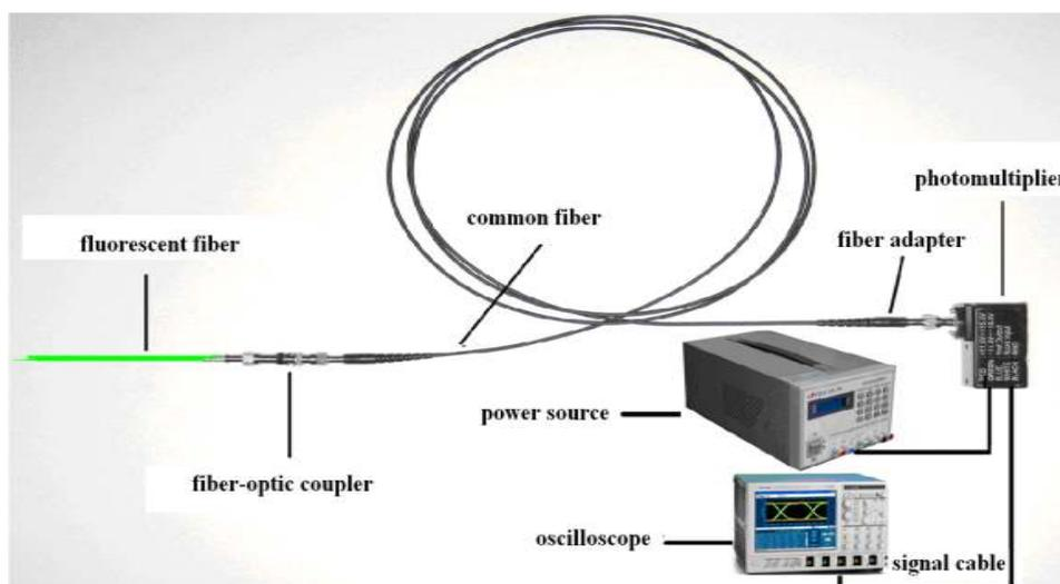
Fig. 2: Image of the fluorescent fiber sensing system
