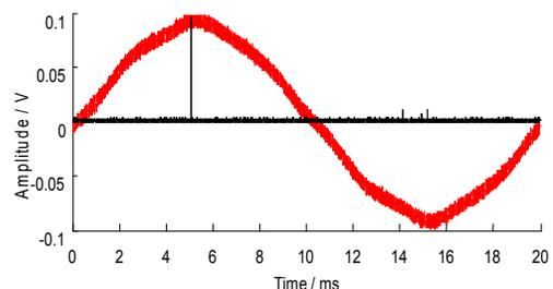
Fig. 6: PD optical pulses in one cycle
