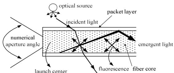
Fig. 1: Optical signals received by fluorescent fiber
