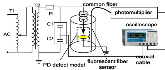
Fig. 3: Experimental platform for PD optical detection in transformer oil
