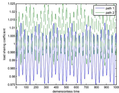
Fig. 9: Load sharing (gear 2 eccentric error)
