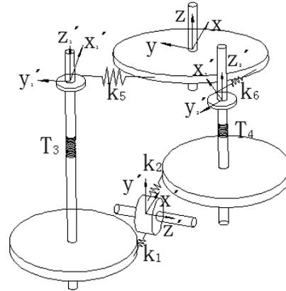
Fig. 2: Split torque mode (damping element, support element not shown)
