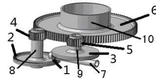
Fig. 1: Face gear split torque transmission
