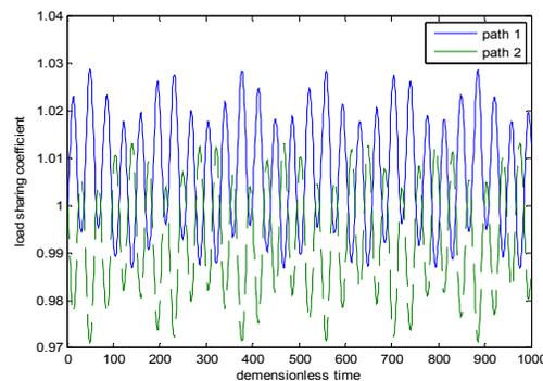
Fig. 12: Load sharing (gear 5 eccentric error)
