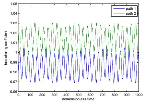
Fig. 11: Load sharing (gear 4 eccentric error)
