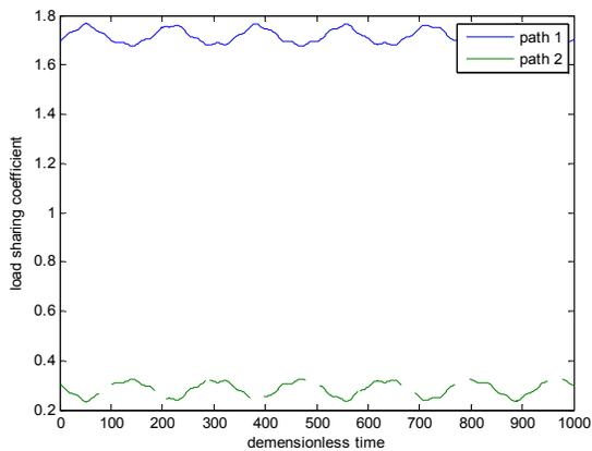
Fig. 3: Load sharing without shaft floating
