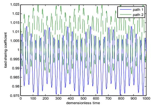
Fig. 10: Load sharing (gear 3 eccentric error)
