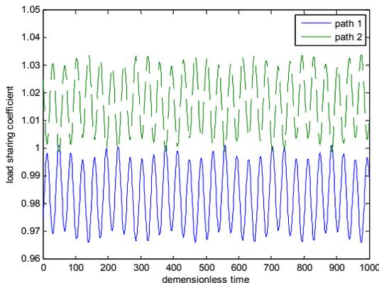
Fig. 15: Load sharing (shaft 2 eccentric error)
