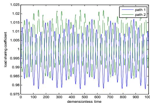
Fig. 13: Load sharing (gear 6 eccentric error)
