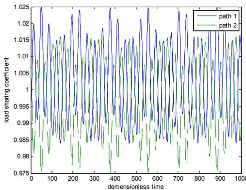
Fig. 8: Load sharing (gear 1 eccentric error)
