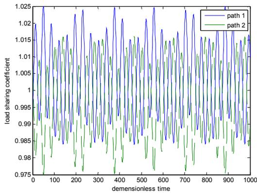
Fig. 14: Load sharing (shaft 1 eccentric error)
