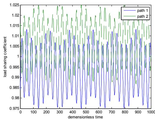
Fig. 16: Load sharing (shaft 3 eccentric error)
