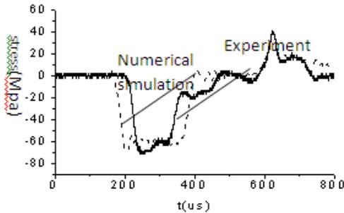
Fig. 9: The curves of incident wave and reflected wave
