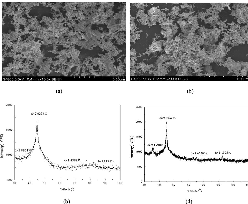
Fig. 1: (a) SEM image of fresh nZVI particles prepared in the presence of 20 kHz ultrasound, (b) SEM image of aged nZVI particles prepared in the presence of 20 kHz ultrasound (360 min), (c) XRD patterns of fresh nZVI particles prepared in the presence of 20 kHz ultrasound and (d) XRD patterns of aged nZVI
