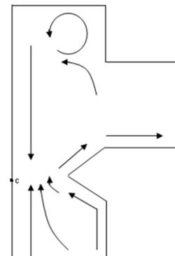
Fig. 8: Internal flow mechanism in CFB with narrowed bed cross section
