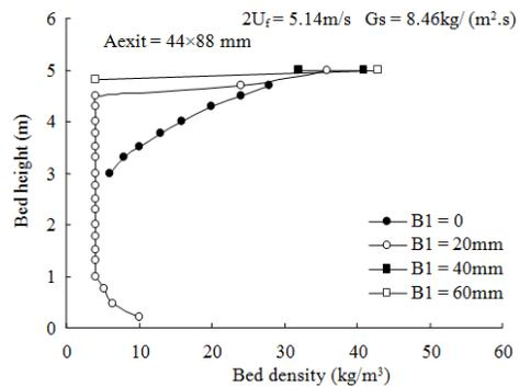
Fig. 6: Influence of  $B$  on bulk density profile (Model 1)
