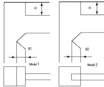
Fig. 5: Narrowed bed exit structures
