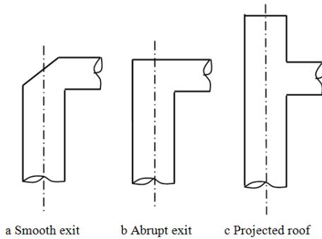
Fig. 2: Three typical exit geometries
