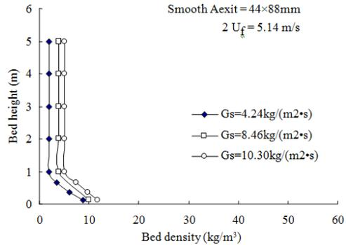
Fig. 3: Bed density profile in CFB with smooth exit
