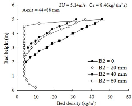
Fig. 7: Influence of  $B$  on bulk density profile (Model 2)
