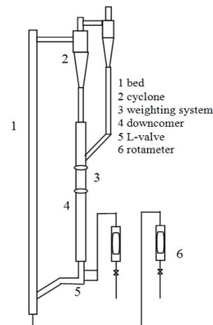
Fig. 1: Schematic diagram of experimental system
