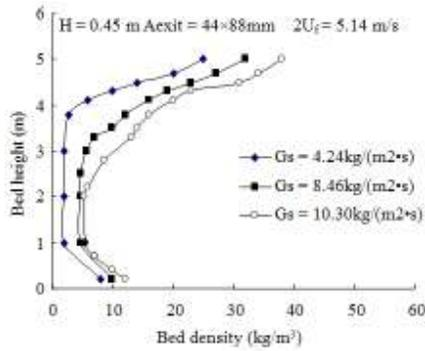
Fig. 4: Bed density profile in CFB with a projected roof
