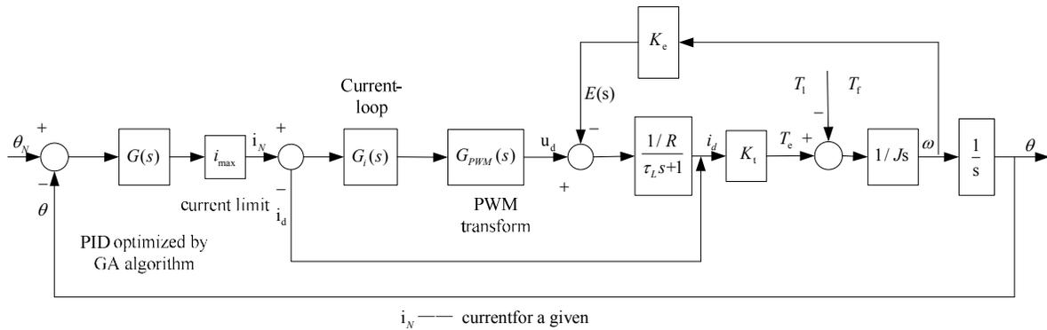
Fig. 3: The position and current double closed-loop structure
