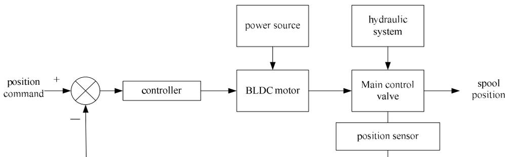
Fig. 1: The structure of the DDA system
