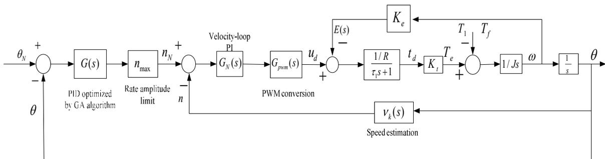
$\theta_N$ —Position given;  $\theta$ — Position feedback;  $n_N$ — Speed given;  $n$ —Speed feedback;  $\tau_1$ —electromagnetic time constant,  $\tau_1 = (L - M) / R$ ;
