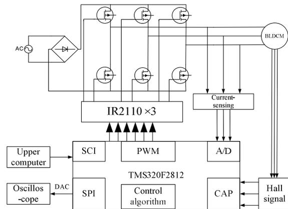
Fig. 5: Schematic of system implementation
