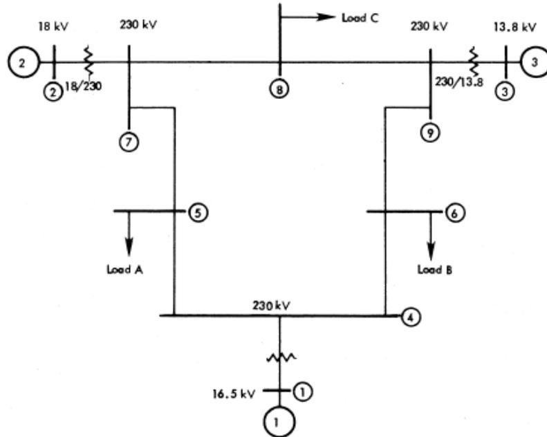
Fig. 2: A 9-bus IEEE testing system
