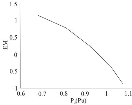
Fig. 3: Change in energy margin with respect to generator power change at bus 2
