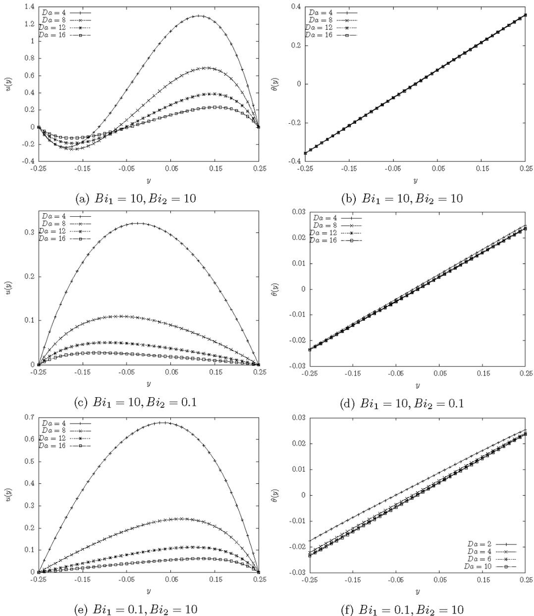
Fig. 4: Velocity profiles and temperature profiles of non-linear, non-Darcy flow for various values of  $Da$  and different combination of Biot numbers,  $Bi_1$  and  $Bi_2$  with  $Br = 0.001, GR = 200$  and  $F = 1$
