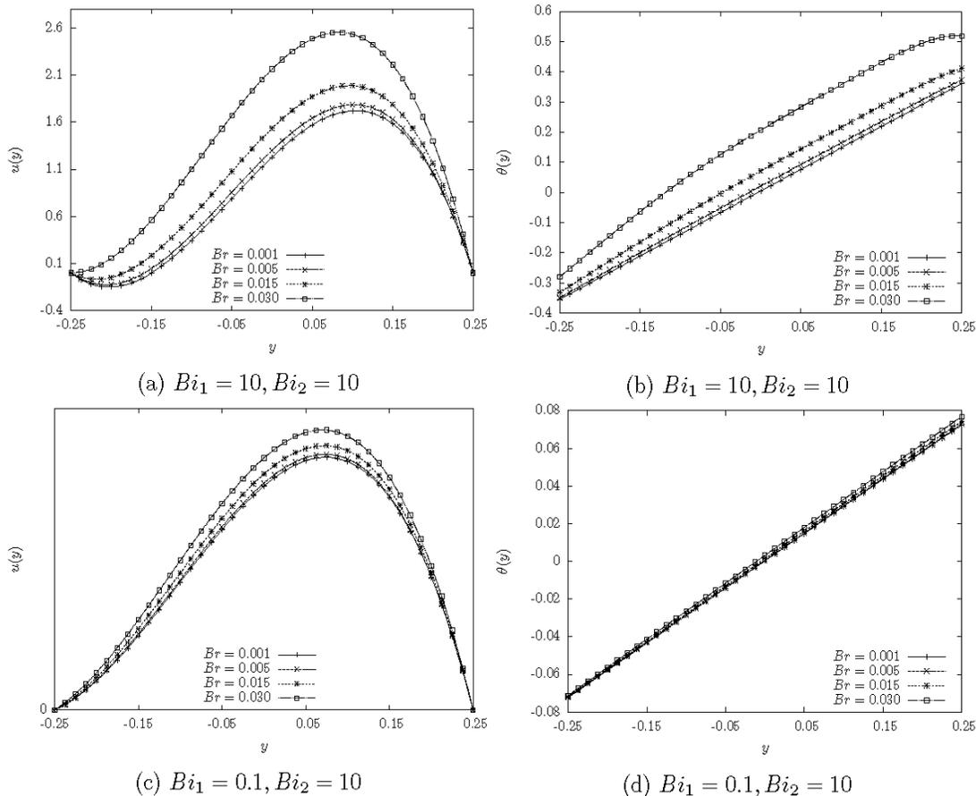
Fig. 3: Velocity profiles and temperature profiles of non-linear, non-Darcy flow for various values of  $Br$  and different combination of Biot numbers,  $Bi_1$  and  $Bi_2$  with  $Br = 0.001, GR = 200$  and  $Da = 2$
