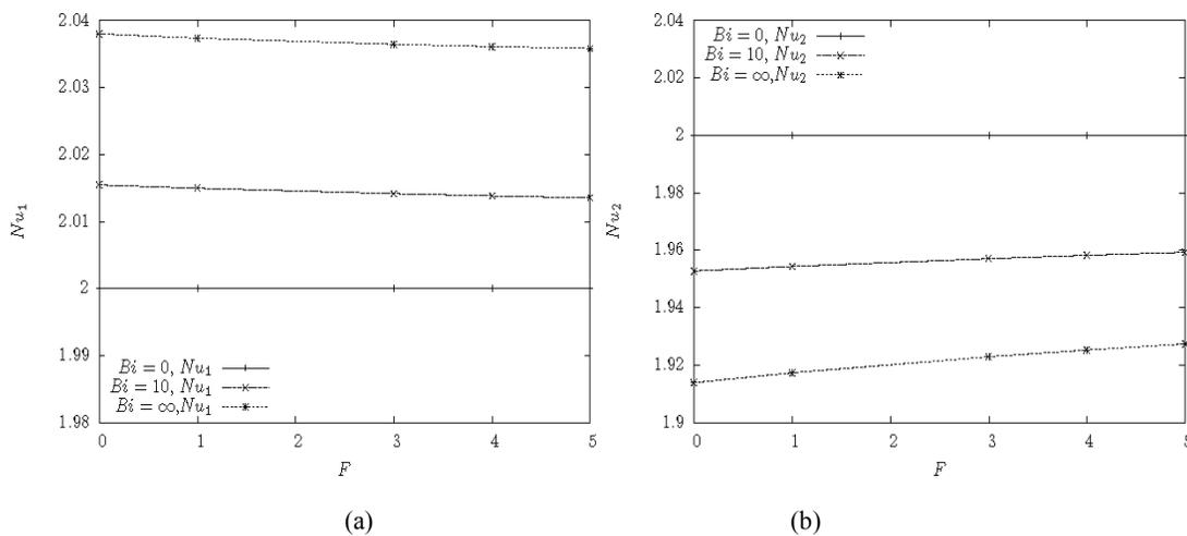
Fig. 11: Effect of Forchheimer drag term ( $F$ ) on Nusselt number values, (a):  $Nu_1$  and (b):  $Nu_2$  for three kinds of boundary conditions on temperature ( $Bi = 0$ -Neumann,  $Bi = 10$ -Robin and  $Bi \rightarrow \infty$ -Dirichlet) where  $Bi_1 = Bi_2 = Bi$ ,  $GR = 200$ ,  $Br = 0.001$  and  $Da = 2$
