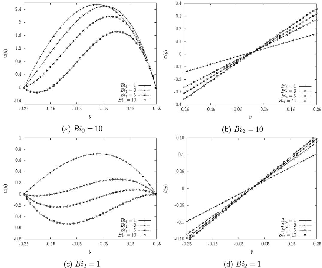
Fig. 6: Velocity profiles and temperature profiles of non-linear, non-Darcy flow for various values of  $Bi_1$  and different variation of  $Bi_2$  with  $GR = 200, Br = 200, Br = 0.001, F = 1$  and  $Da = 2$
