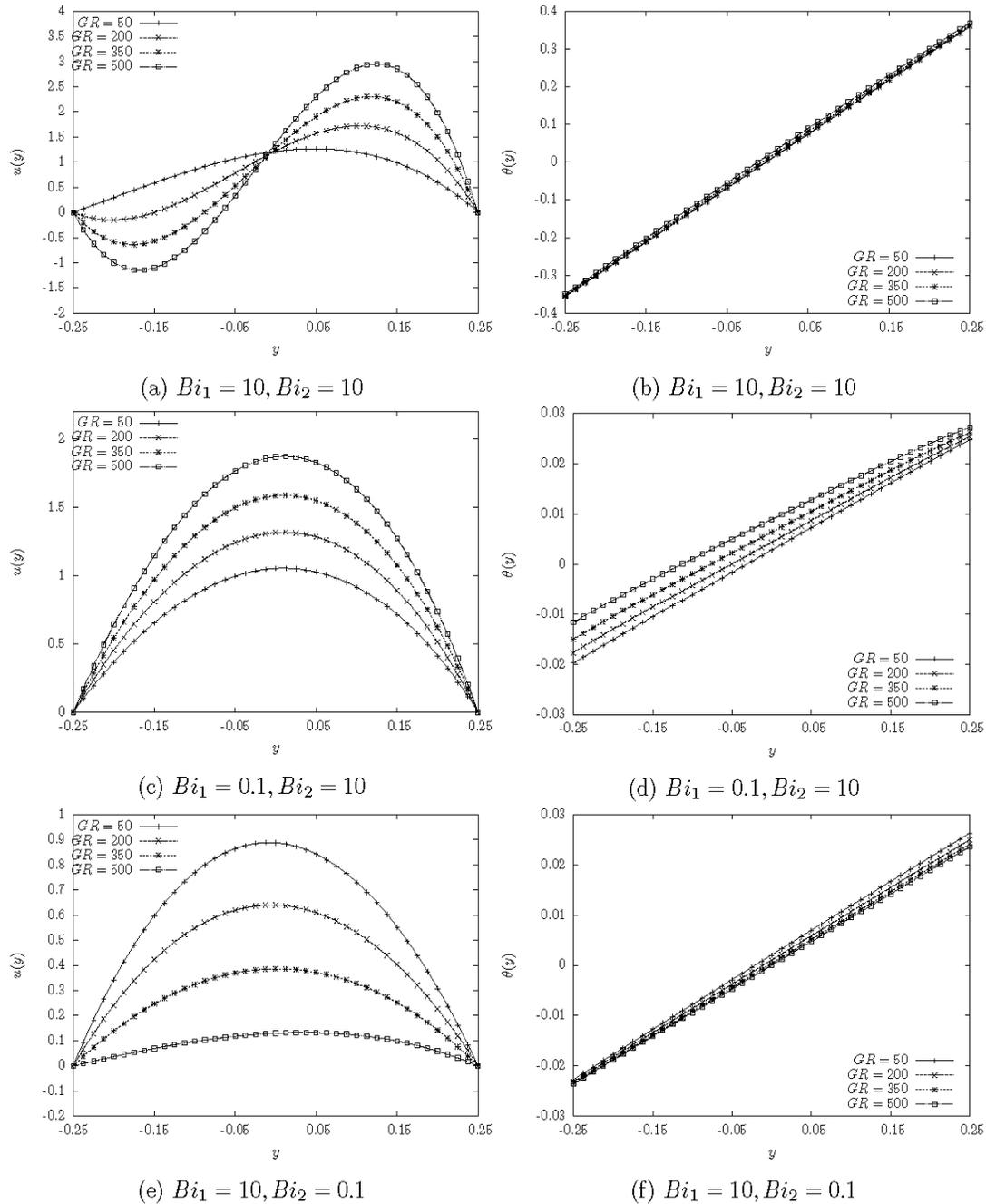
Fig. 2: Velocity profiles (left) and temperature profiles (right) of non-linear, non-Darcy flow for various values of  $GR$  and different combination of Biot numbers,  $Bi_1$  and  $Bi_2$  with  $Br = 0.001, F = 1$  and  $Da = 2$
