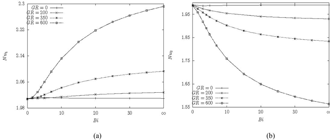
Fig. 14: Effect of Biot numbers  $Bi$  (where  $Bi_1 = Bi_2 = Bi$ ), on Nusselt number values, (a):  $Nu_1$  and (b):  $Nu_2$  for various mixed convection parameter  $GR$ , with  $Da = 2$ ,  $Br = 0.001$  and  $F = 1$
