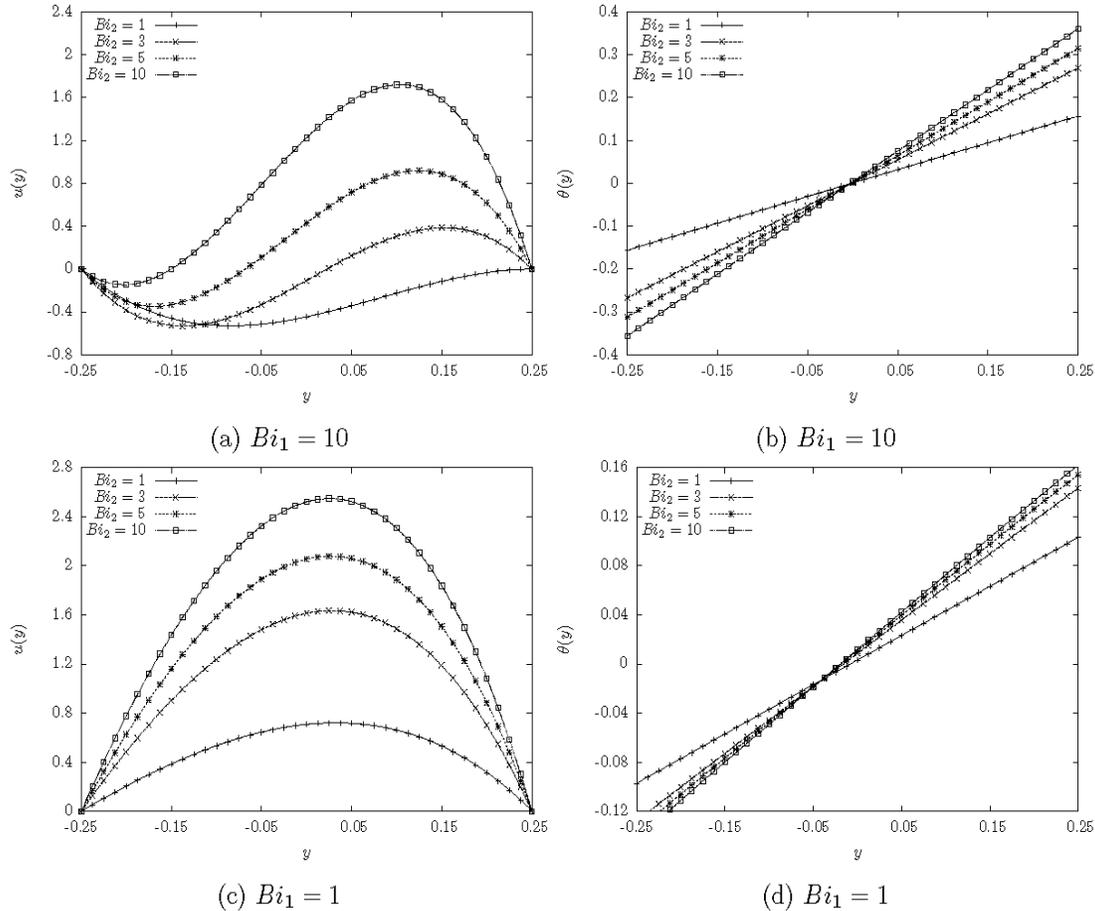
Fig. 7: Velocity profiles and temperature profiles of non-linear, non-Darcy flow for various values of  $Bi_2$  and different variation of  $Bi_1$  with  $GR = 200, Br = 0.001, F = 1$  and  $Da = 2$
