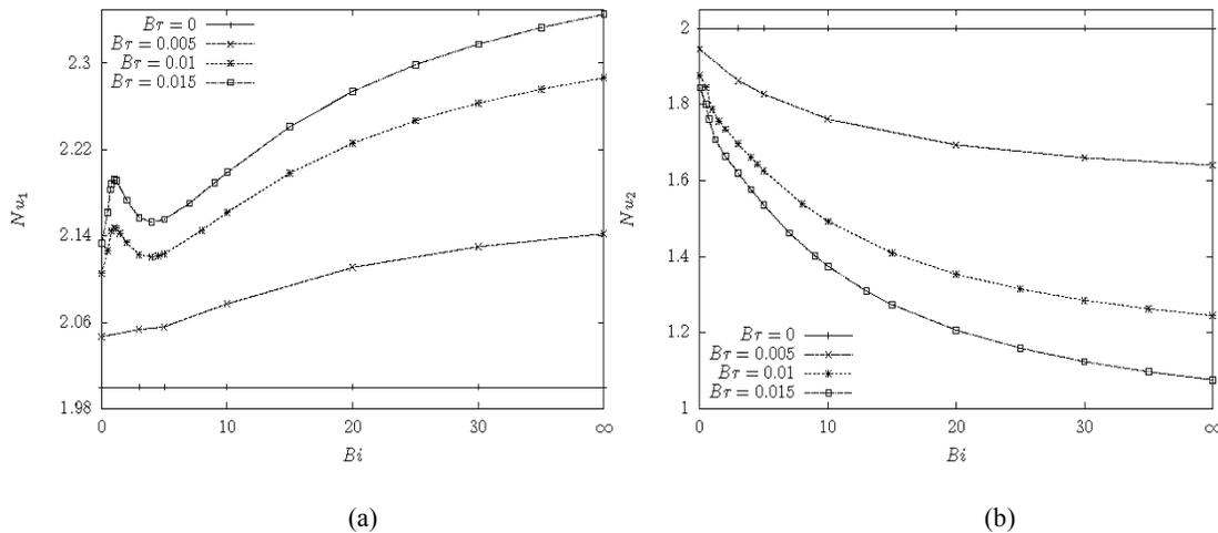
Fig. 15: Effect of Biot numbers  $Bi$  (where  $Bi_1 = Bi_2 = Bi$ ), on Nusselt number values, (a):  $Nu_1$  and (b):  $Nu_2$  for various values of Brinkman number  $Br$ , with  $Da = 2$ ,  $GR = 200$  and  $F = 1$
