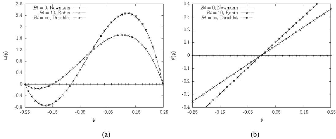
Fig. 8: (a) Velocity profile and (b) temperature profile of non-linear, non-Darcy flow for three kinds of boundary conditions on temperature ( $Bi = 0$ -Neumann,  $Bi = 10$ -Robin and  $Bi \rightarrow \infty$ -Dirichlet) where  $Bi_1 = Bi_2 = Bi, GR = 200, Br = 0.001, F = 1$  and  $Da = 2$
