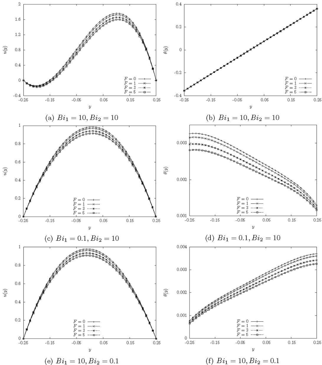
Fig. 5: Velocity profiles and temperature profiles of non-linear, non-Darcy flow for various values of  $F$  and different combination of Biot numbers,  $Bi_1$  and  $Bi_2$  with  $GR = 200, Br = 0.001$  and  $Da = 2$
