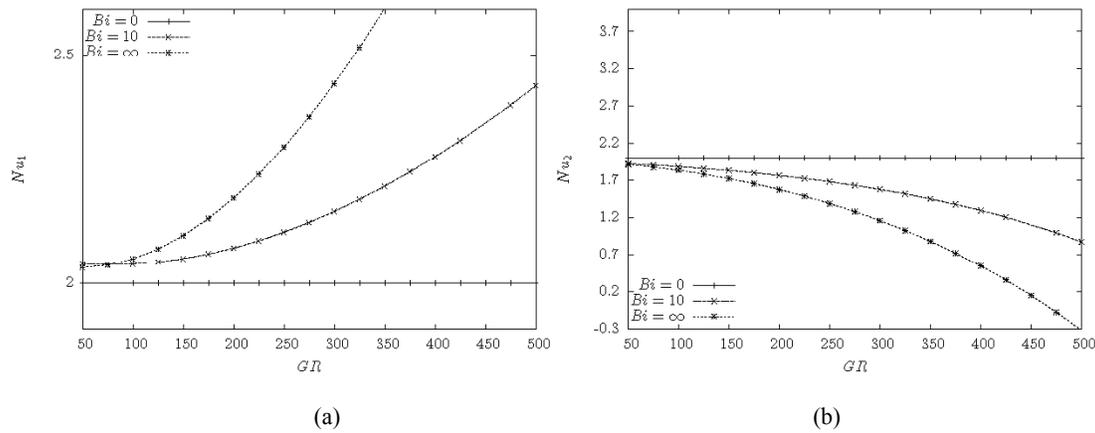
Fig. 9: Effect of mixed convection parameter ( $GR$ ) on Nusselt number values, (a)  $Nu_1$  and (b)  $Nu_2$  for three kinds of boundary conditions on temperature ( $Bi = 0$ -Neumann,  $Bi = 10$ -Robin and  $Bi \rightarrow \infty$ -Dirichlet) where  $Bi_1 = Bi_2 = Bi, Br = 0.001, F = 1$  and  $Da = 2$
