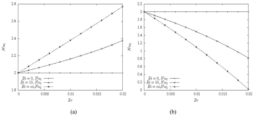
Fig. 10: Effect of viscous dissipation ( $Br$ ) on Nusselt number values, (a):  $Nu_1$  and (b):  $Nu_2$  for three kinds of boundary conditions on temperature ( $Bi = 0$ -Neumann,  $Bi = 10$ -Robin and  $Bi \rightarrow \infty$ -Dirichlet) where  $Bi_1 = Bi_2 = Bi$ ,  $GR = 200$ ,  $F = 1$  and  $Da = 2$
