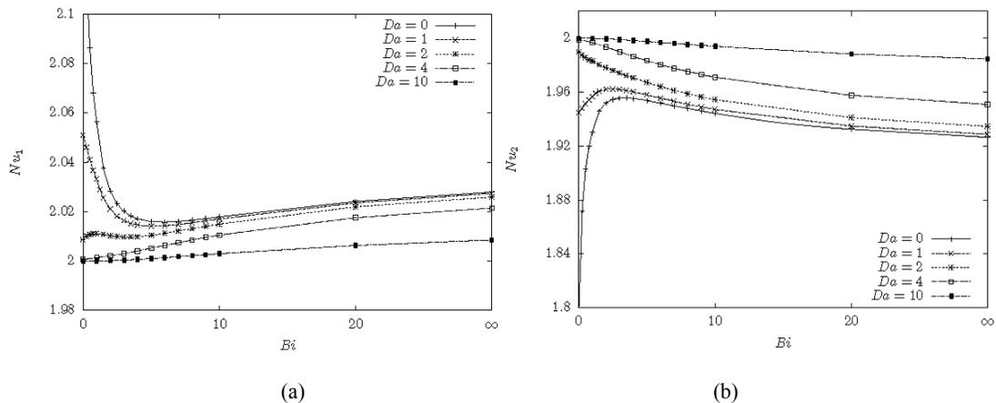
Fig. 13: Effect of Biot numbers  $Bi$  (where  $Bi_1 = Bi_2 = Bi$ ), on Nusselt number values, (a):  $Nu_1$  and (b):  $Nu_2$  for various Darcy numbers  $Da$ , with  $GR = 200$ ,  $Br = 0.001$  and  $F = 1$
