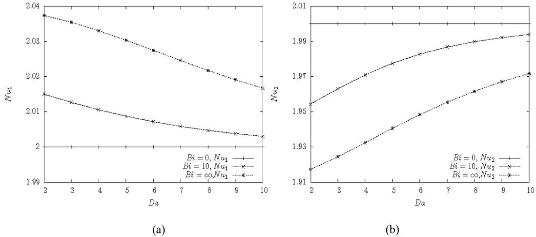
Fig. 12: Effect of Darcy number ( $Da$ ) on Nusselt number values, (a):  $Nu_1$  and (b):  $Nu_2$  for three kinds of boundary conditions on temperature ( $Bi = 0$ -Neumann,  $Bi = 10$ -Robin and  $Bi \rightarrow \infty$ -Dirichlet) where  $Bi_1 = Bi_2 = Bi$ ,  $GR = 200$ ,  $Br = 0.001$  and  $F = 1$
