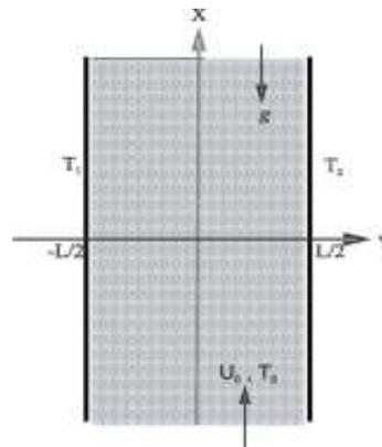
Fig. 1: Physical configuration of vertical channel containing fully-developed mixed convection non-linear, non-Darcy flow
