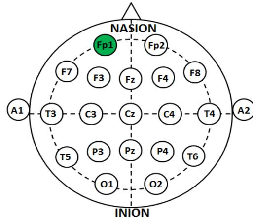
Fig. 1: Fp1 electrode placement in the 10-20 international system
