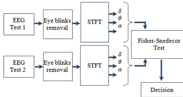
Fig. 2: Flowchart of our methodology to illustrate effects of changing difficulty levels on the prefrontal brain area during a learning task
