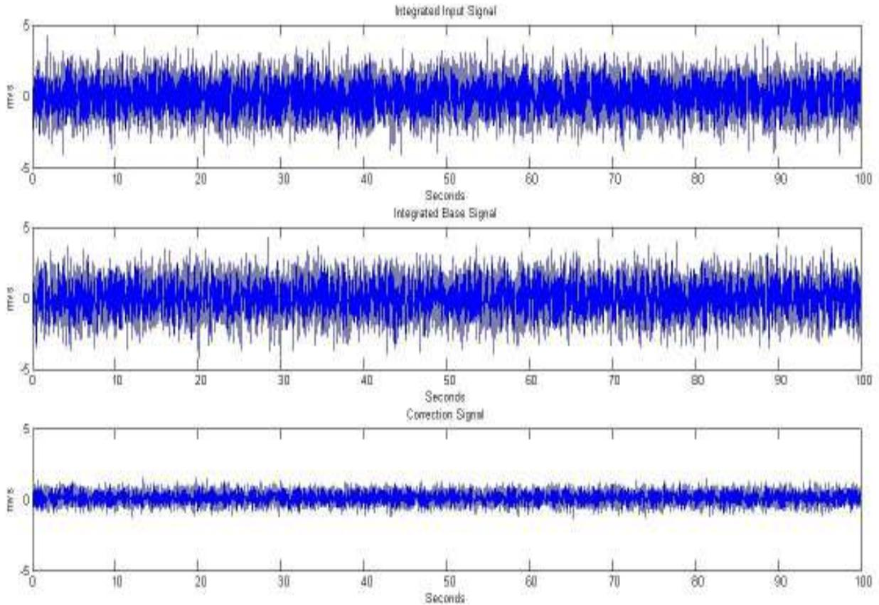
Fig. 6: Integration drift for 100 seconds
