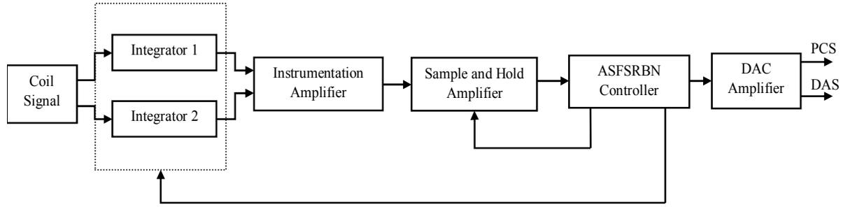
Fig. 1: FPGA based block diagram of the integrator system
