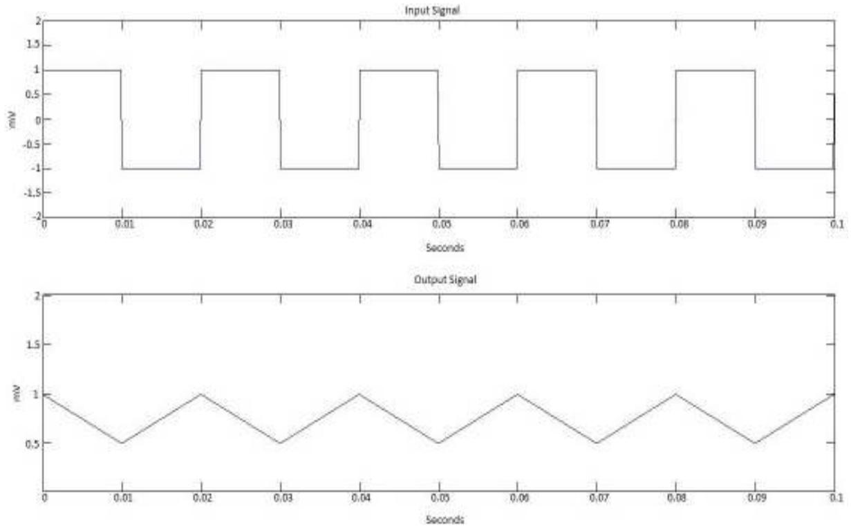
Fig. 5: Integrator test from the input signal
