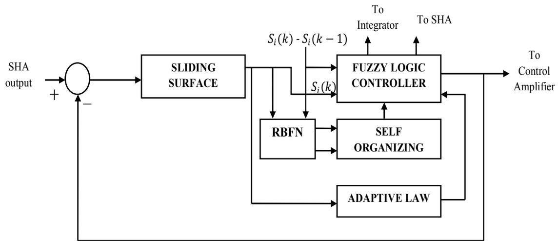
Fig. 4: FPGA based adaptive self optimized fuzzy sliding mode radial basis function neural network (ASFSRBN) controller
