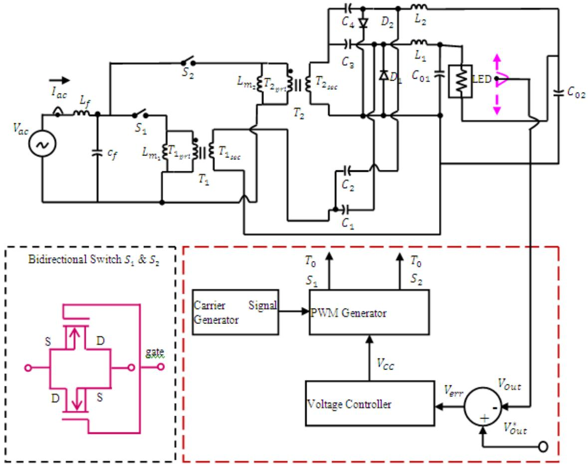
Fig. 2: Overall proposed BL isolated interleaved zeta converter
