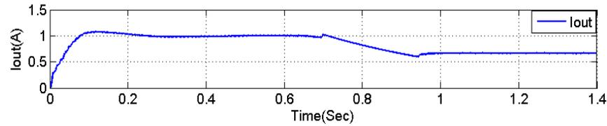
Fig. 9b: Converter output current response when sudden change in rated output voltage
