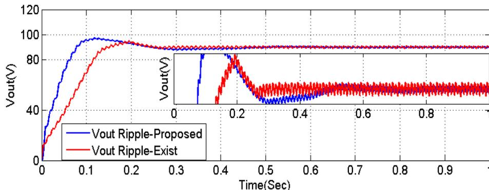
Fig. 8: Ripple factor response of the proposed BL Interleaved converter and the existing bridge converter
