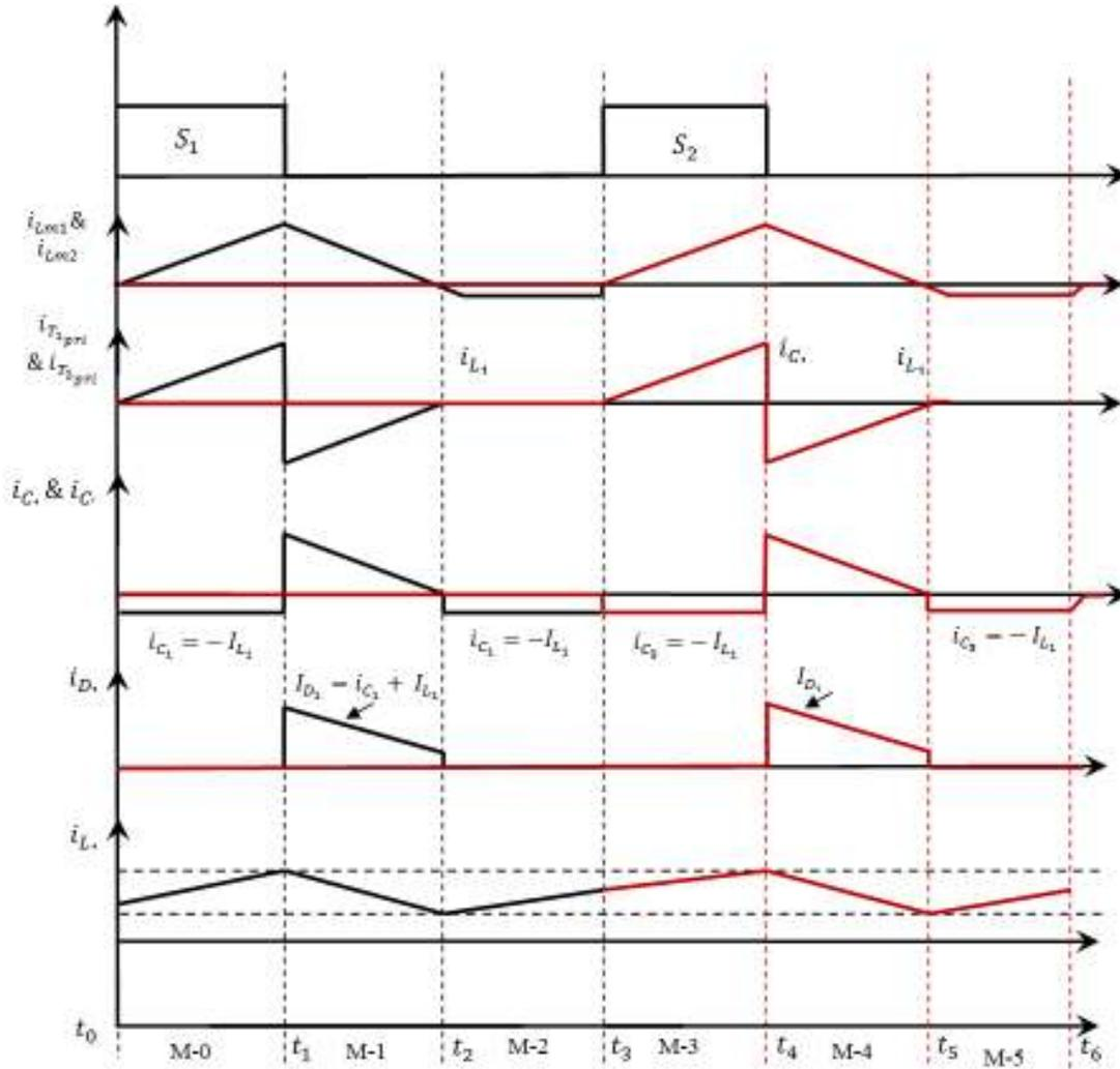
Fig. 5: Theoretical analysis waveform
