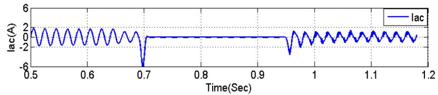
Fig. 9c: Supply current response when sudden change in rated output voltage
