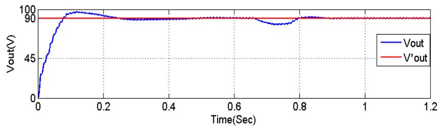
Fig.10b: Response of the converter output voltage
