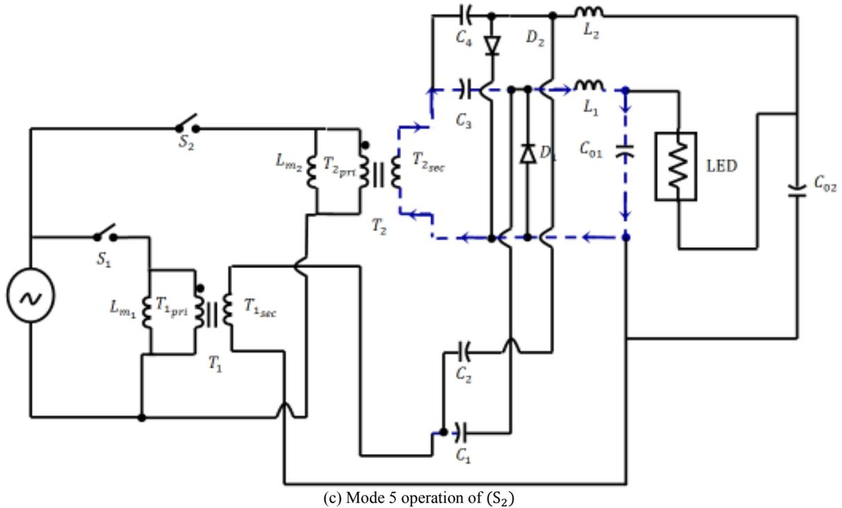
Fig. 4: Conduction modes of switch S<sub>2</sub> during positive cycle
