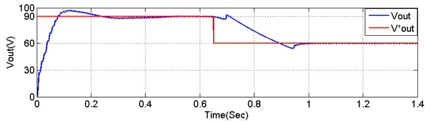
Fig. 9a: Converter output voltage response when sudden change in rated output voltage
