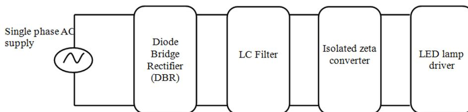
Fig. 1: Conventional DBR based isolated zeta converter
