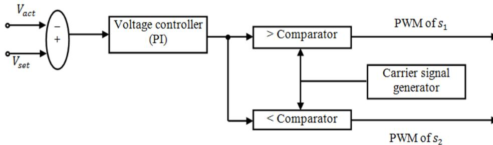
Fig. 6: Proposed converter based LED drive voltage control loop
