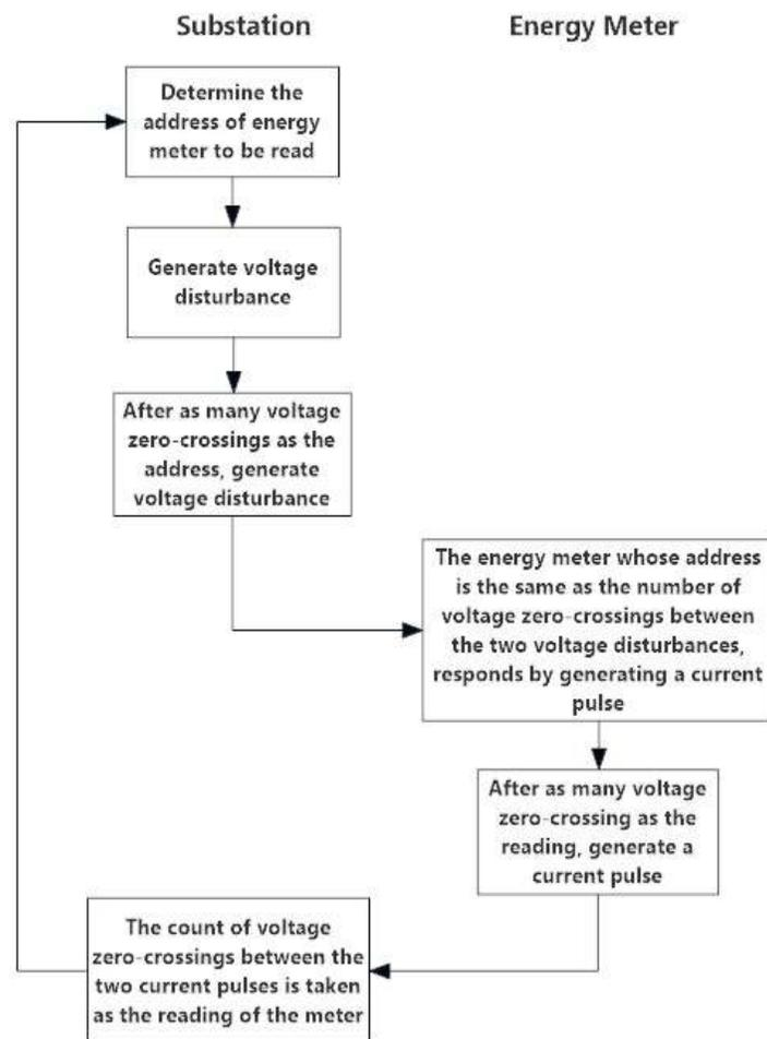
Fig. 13: Flow chart showing sequence of interactions between substation and energy meters
