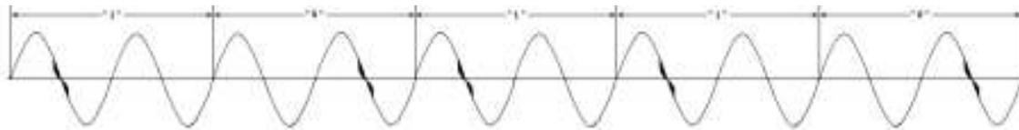
Fig. 3: TWACS outbound signal for bit pattern "10110"
