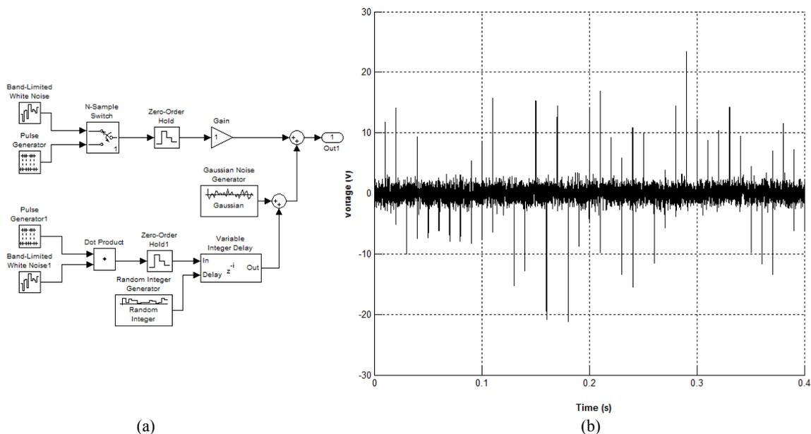
Fig. 11: Power line noise model, (a) SIMULINK model, (b) noise waveform
