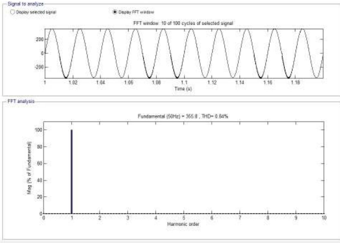
Fig. 14: Voltage harmonics in TWACS outbound signal
