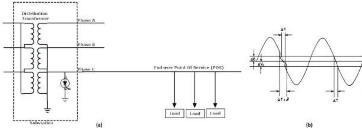
Fig. 1: TWACS outbound signal generation, (a) schematic diagram, (b) voltage waveform
