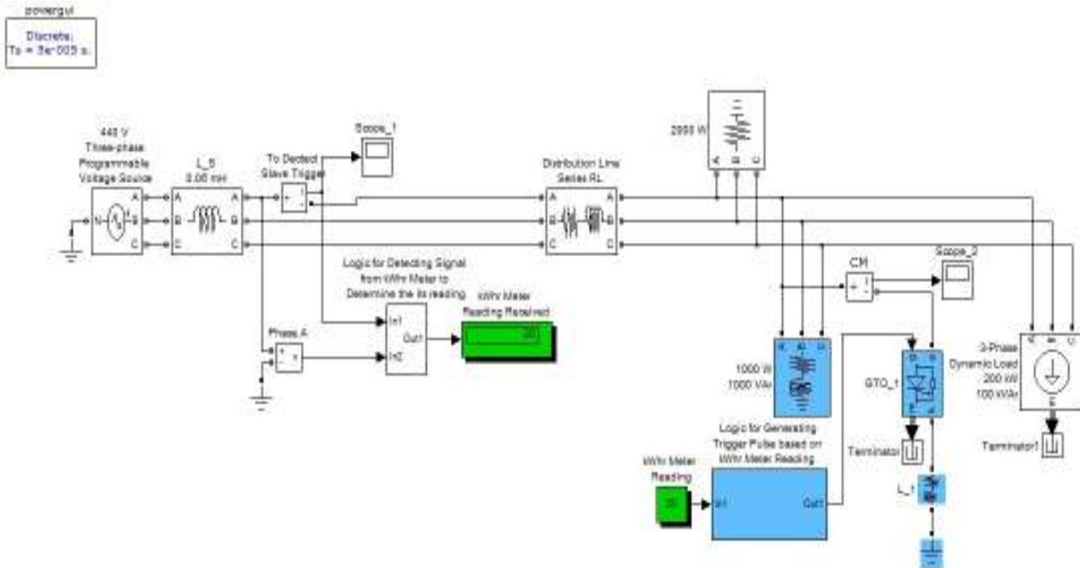
Fig. 12: SIMULINK model for energy meter reading transmission
