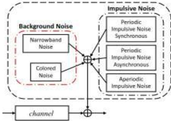
Fig. 10: Classification of power line noise
