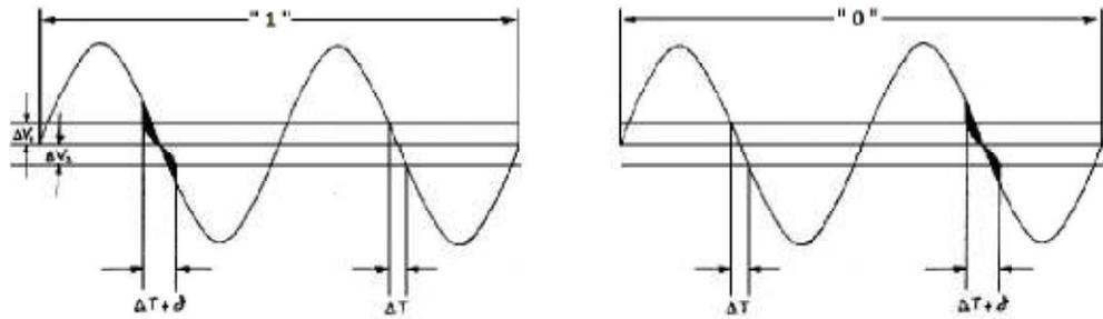
Fig. 2: TWACS outbound signal-bit definitions
