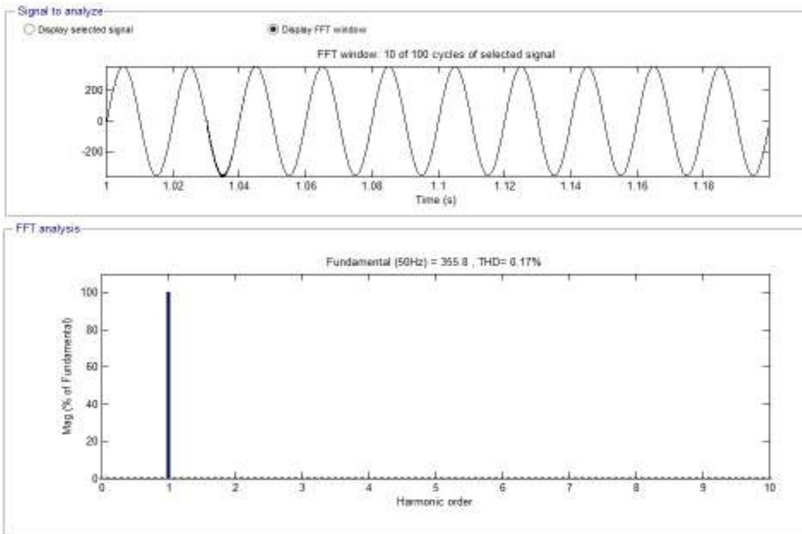
Fig. 15: Voltage harmonics in the proposed outbound signal
