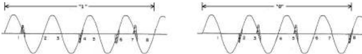
Fig. 6: TWACS inbound signal-bit patterns
