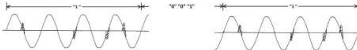
Fig. 7: TWACS inbound signal for bit pattern "10011"
