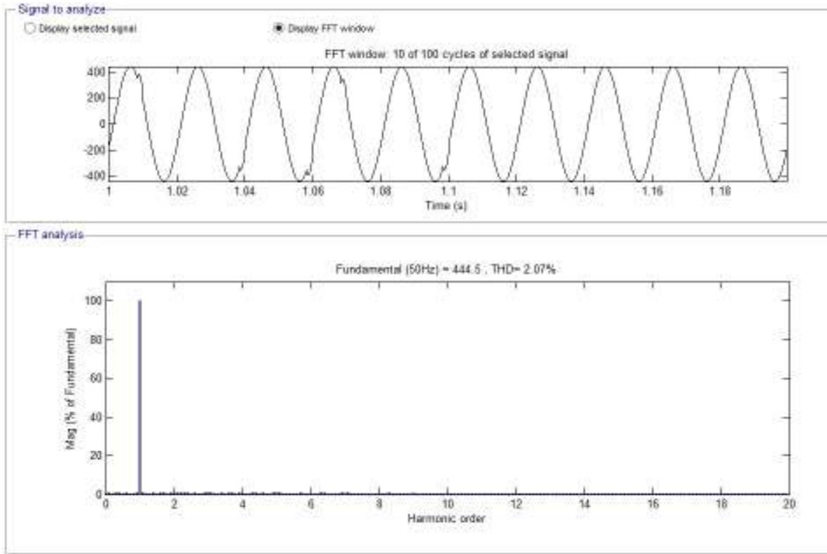
Fig. 16: Current harmonics in TWACS inbound signal
