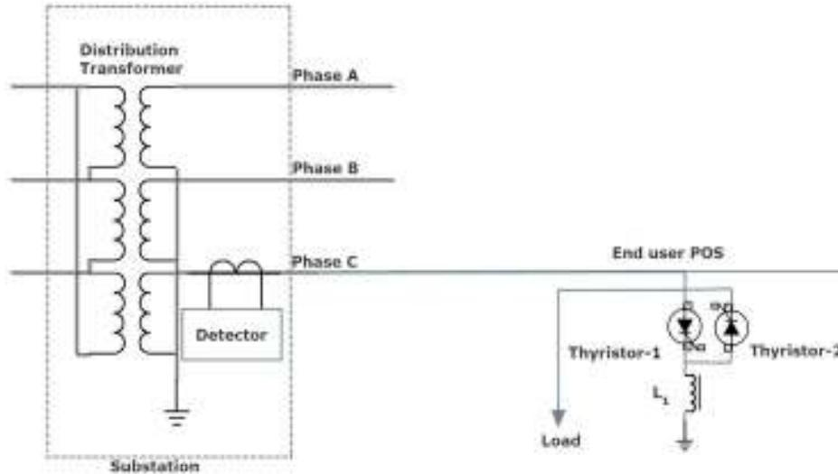
Fig. 5: TWACS inbound signal generation-schematic diagram
