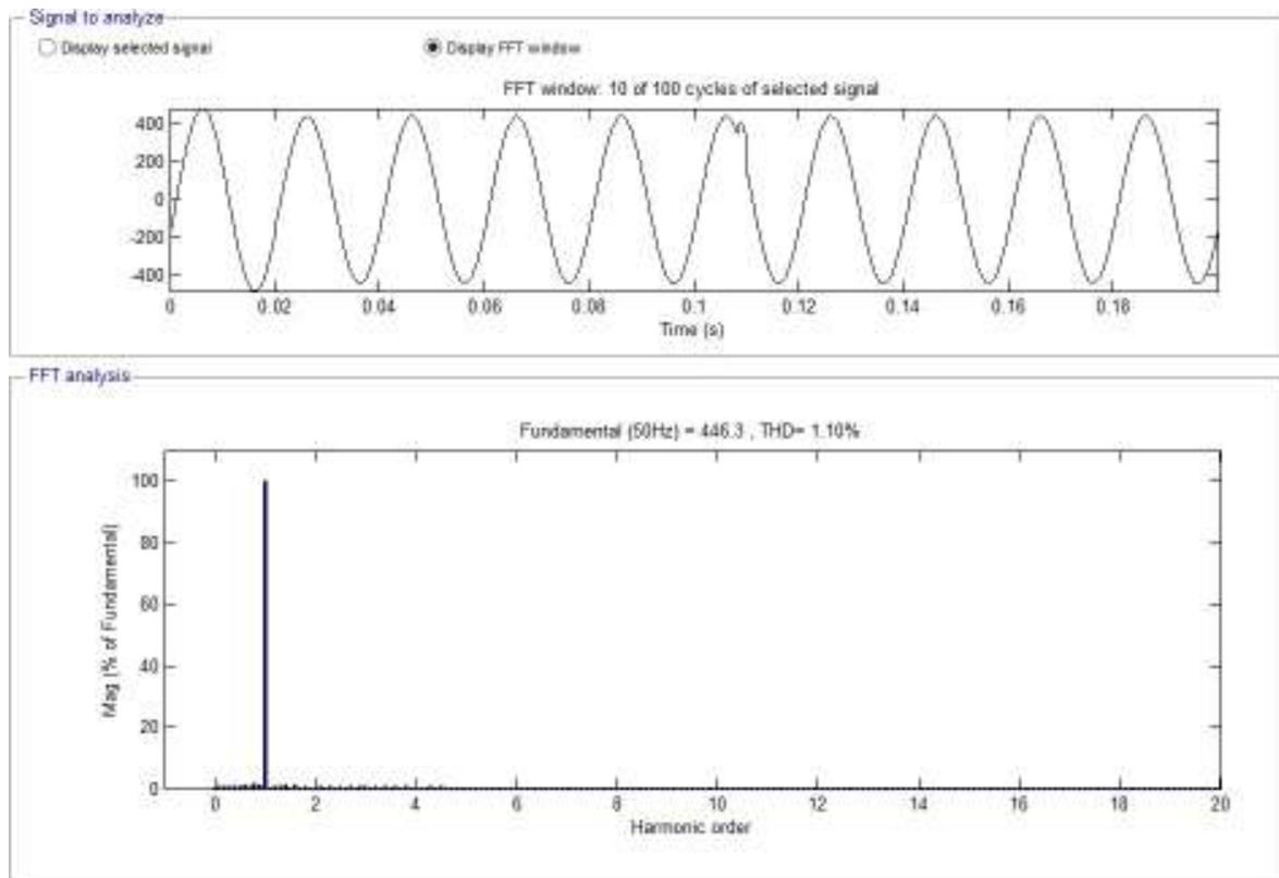
Fig. 17: Current harmonics in the proposed inbound signal
