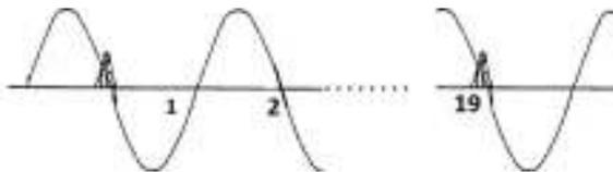
Fig. 8: Proposed inbound signal for decimal 19
