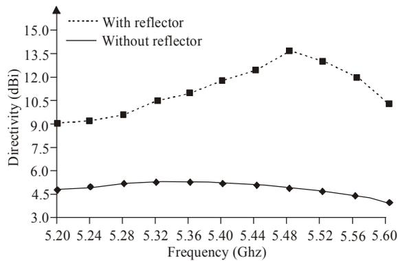
Fig. 6: Simulated peak directivity gain of the CDRA with and without reflector
