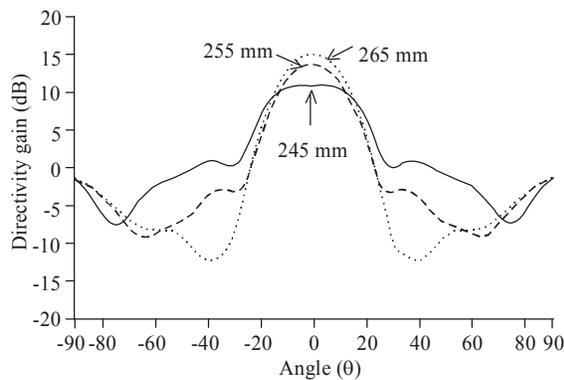
Fig. 7: Effect of diameter of the reflector on the directivity gain of the antenna
