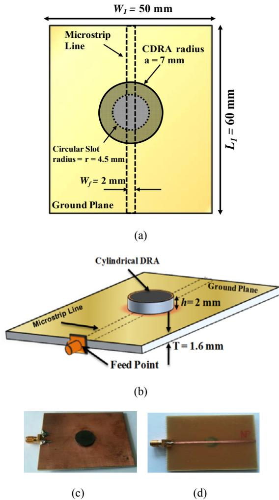
Fig. 1: (a) Geometry of CDRA, (b) perspective view of CDRA, (c) front view of fabricated CDRA, (d) back view of fabricated
