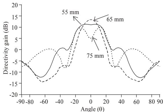
Fig. 8: Effect of reflector depths on the directivity gain of the antenna
