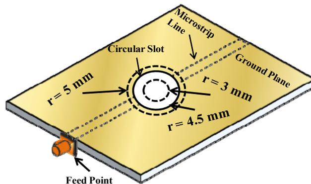
Fig. 10: Geometry of CDRA with different slot radii
