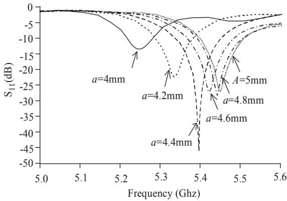
Fig. 11: Effect of different slot radii on the resonance frequency of the CDRA feeder
