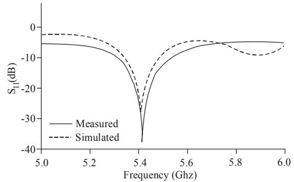
Fig. 3: Simulated and measured return loss ( $S_{11}$ )
