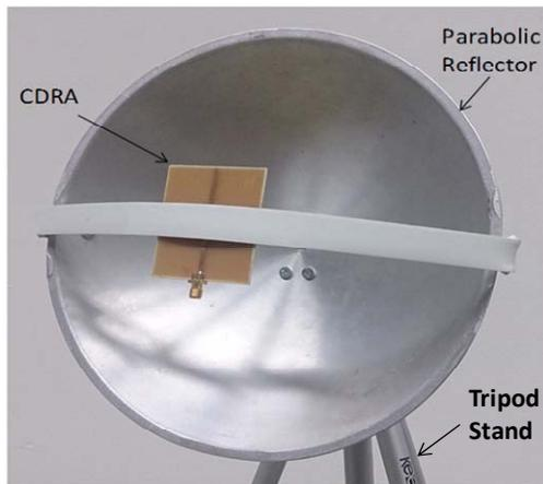
Fig. 2: (a) Geometry of CDRA with parabolic reflector, (b) fabricated CDRA with parabolic reflector
