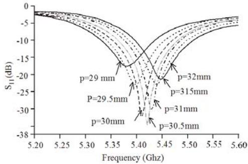
Fig. 14: Effect of different slot positions on the resonance frequency of the CDRA feeder
