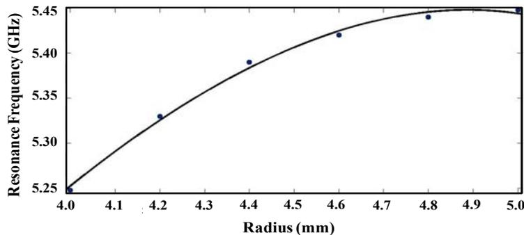
Fig. 12: Plot of resonance frequency versus radius of the slot using curve fitting tool
