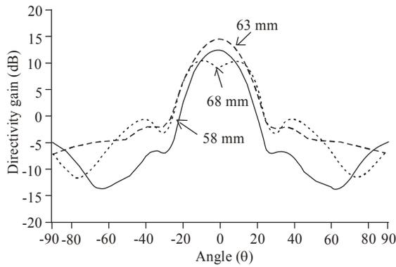
Fig. 9: Effect of focal point of the reflector on the directivity gain of the antenna
