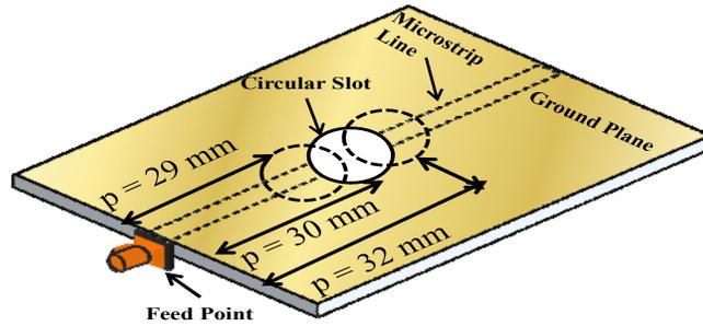
Fig. 13: Geometry of the CDRA showing different positions of the slot
