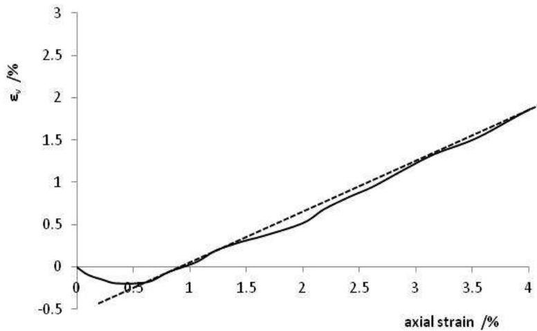
Fig. 4: Volumetric change vs. axial strain
