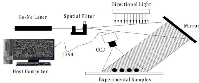
Fig. 1: Illumination and image capture experimental system
