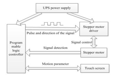
Fig. 1: System structure diagram
