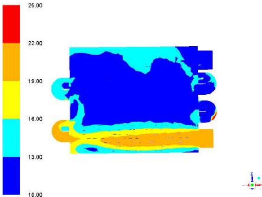
Fig. 5: Contours of total pressure in an XZ plane in the middle of the Y axis (Pascal)
