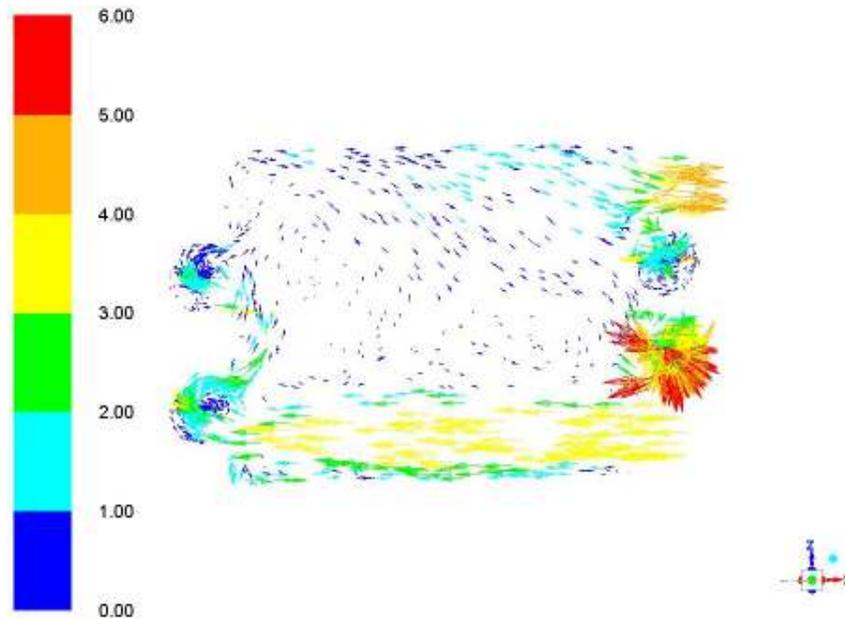
Fig. 4: Velocity vectors (m/s) in an XZ plane in the middle of the Y axis.
