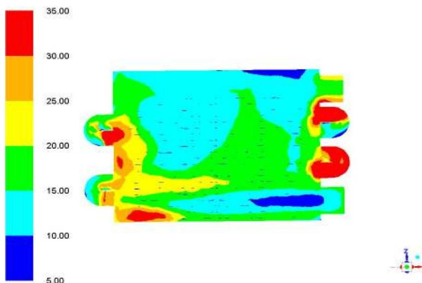
Fig. 6: Contours of turbulence intensity in an XZ plane in the middle of the Y axis (%)
