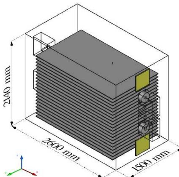
Fig. 1: Geometry of the tray dryer. The yellow squares are the air inlet and outlet
