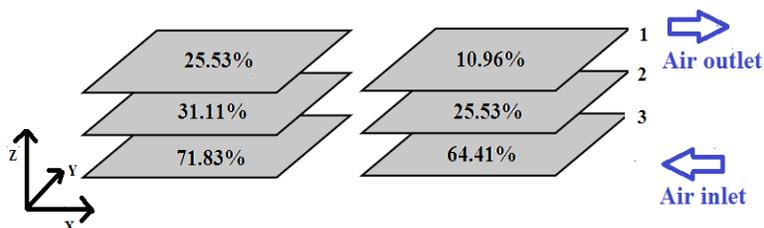
Fig. 2: Schematic of the moisture percentage results at different points of the equipment. The arrows represent the air inlet and outlet. The numbers identify the level which the trays are located
